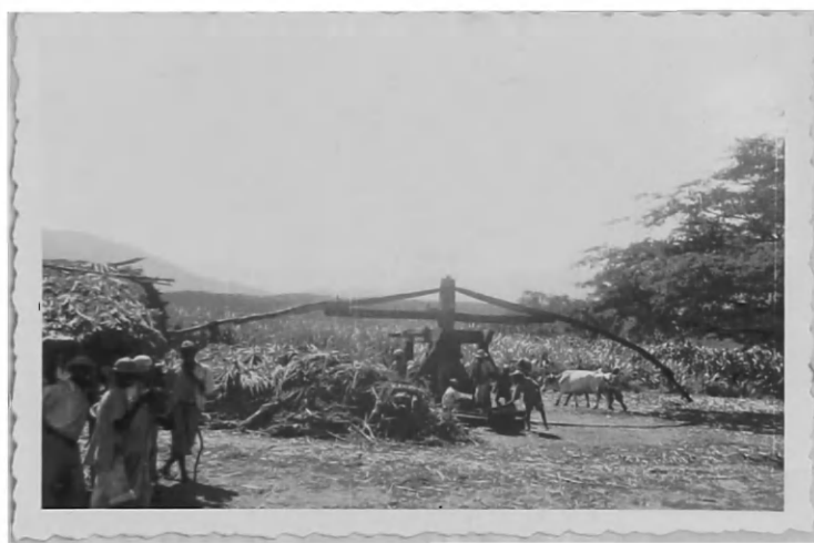
PLATE XXXIII. PRIMITIVE SUGAR-CANE MILLS IN RURAL HAITI. (Upper: a hand press of the most primitive type. Lower: a more modern press which is operated by ox power. This type is most popular in rural Haiti.)
