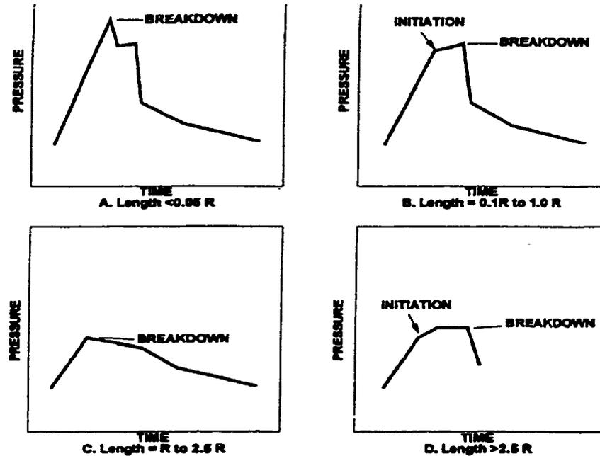
Figure 2.16 Effect of pre-existing crack length (Ishijima and Roegiers, 1983).
