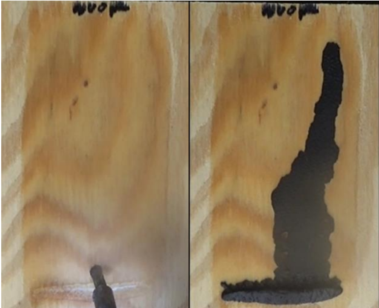
Figure 7.5. Sample of 50/50 TMPTE/TEGDVE with 0.5 phr IOC-8, 1 phr Luperox 231, and 5 wt% fumed silica in a 500 \mu\text{m} layer on pine wood. The resin with exposed grain is shown on the left with the cured polymer after FP on the right.
