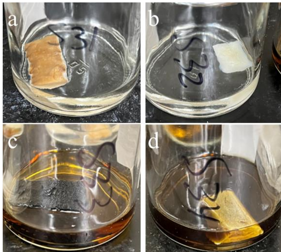
Figure 4.13. Hybrid acrylate and epoxy or vinyl ether polymers of mixed functionality produced by FP submerged in DCM to dissolve linear components. Solutions shown are a) TMPTE/HA; b) TMPTA/PTBGE; c) TEGDVE/HA; d) TMPTA/D12VE.
