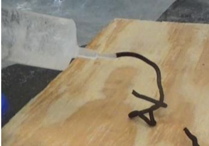
Figure 7.1. 3D printing using manual extrusion of an epoxy-vinyl ether resin from a syringe, with a visible front. The dark material is polymer while the colorless material is uncured resin.
