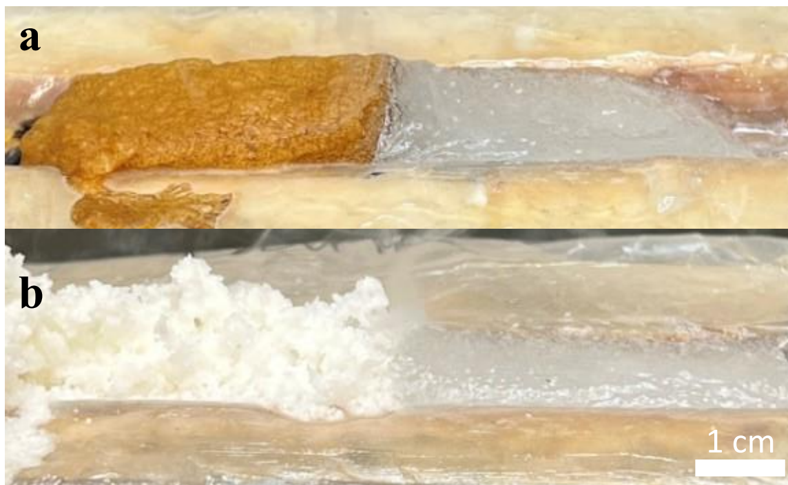
Figure 4.1. Comparison of polymer properties between formulations containing (a) TMPTE with 1 phr IOC-8 and 1 phr L231 with 10 wt% fumed silica and (b) TMPTA with 1 phr L231 and 10 wt% fumed silica, both with an ongoing front.
