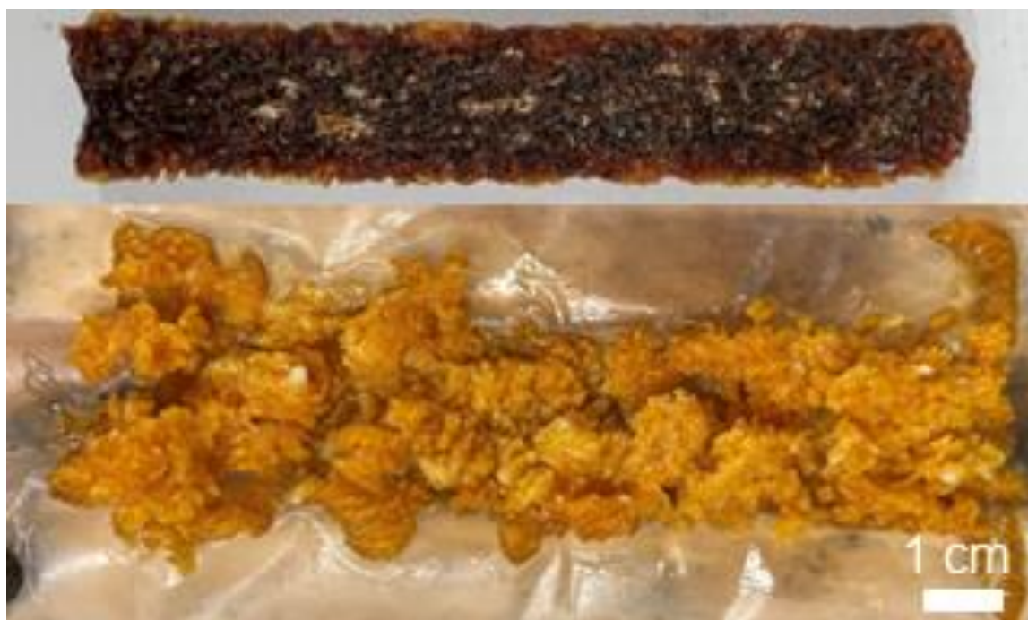
Figure 6.9. Example of material produced with pure TEGDVE (top) and DVE-1,4 (bottom), both containing 0.1 phr IOC-8.
