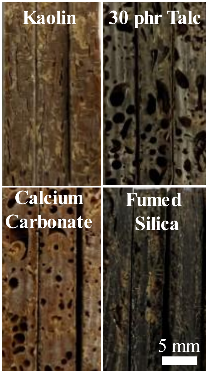
Figure 5.33. Cross section of composite sheets filled with specified filler with noticeable voids in calcium carbonate and talc.
