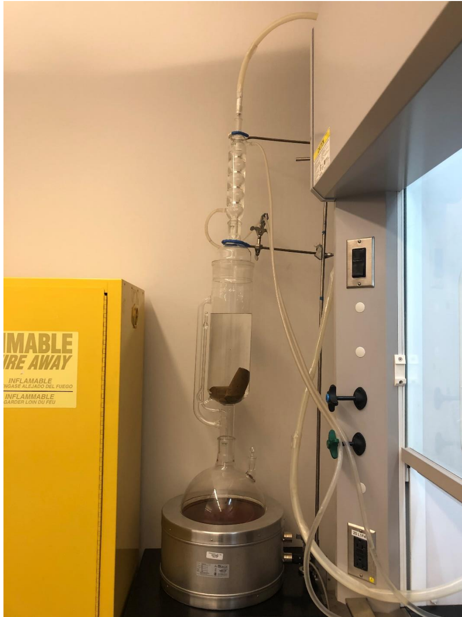
Figure 3. 5. Giant Soxhlet Extractor Cleaning Multiple Large Core Samples in LSU PETE EOR Lab
