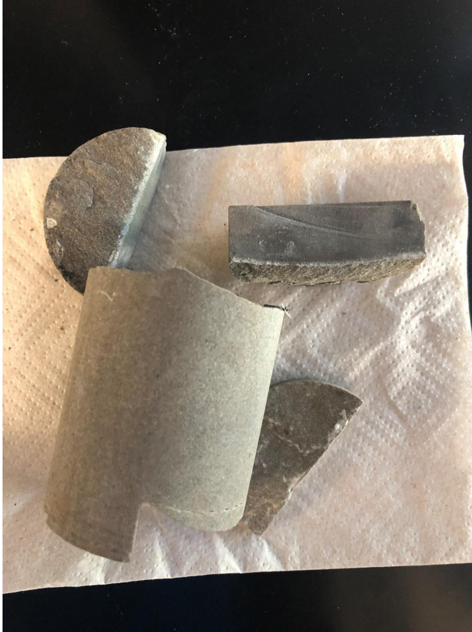
Figure 4. 5. Unconventional Core Samples Fragile After Core Flooding and Gas Injection Experiment at Reservoir Temperature (260 °F)
