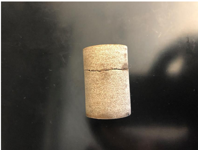
Figure 4. 4. Unconventional Core Samples Fragile During Gas Injection Experiment
