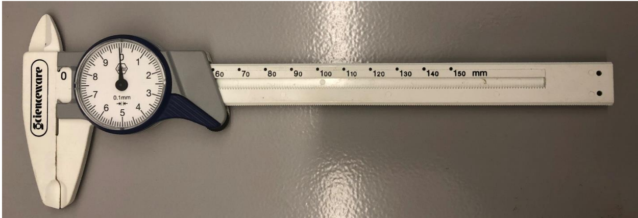
Figure 3. 9. A 0.1 mm Accurate Caliper Used to Determine the Core Plugs and Samples Dimensions
