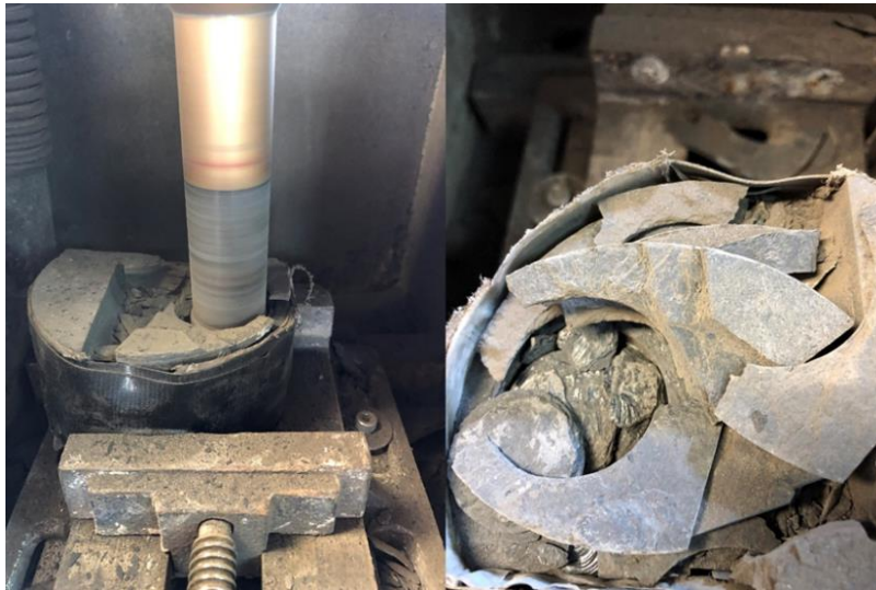
Figure 4.1. Unconventional Core Samples Fragile While Cutting
