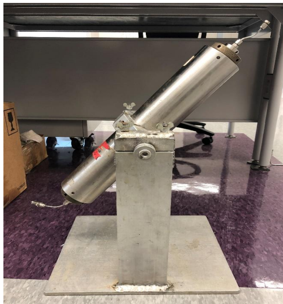
Figure 3. 13. A 500 mL Capacity Fluid Injection Transfer Vessel Used to Flood the Cores with the Oil
