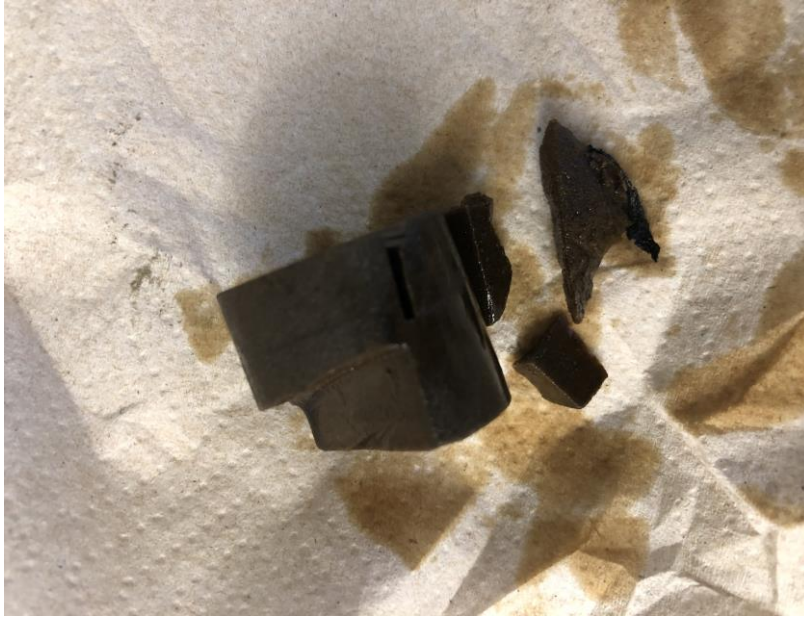
Figure 4. 3. Unconventional Core Samples Fragile During Oil Flooding Experiment
