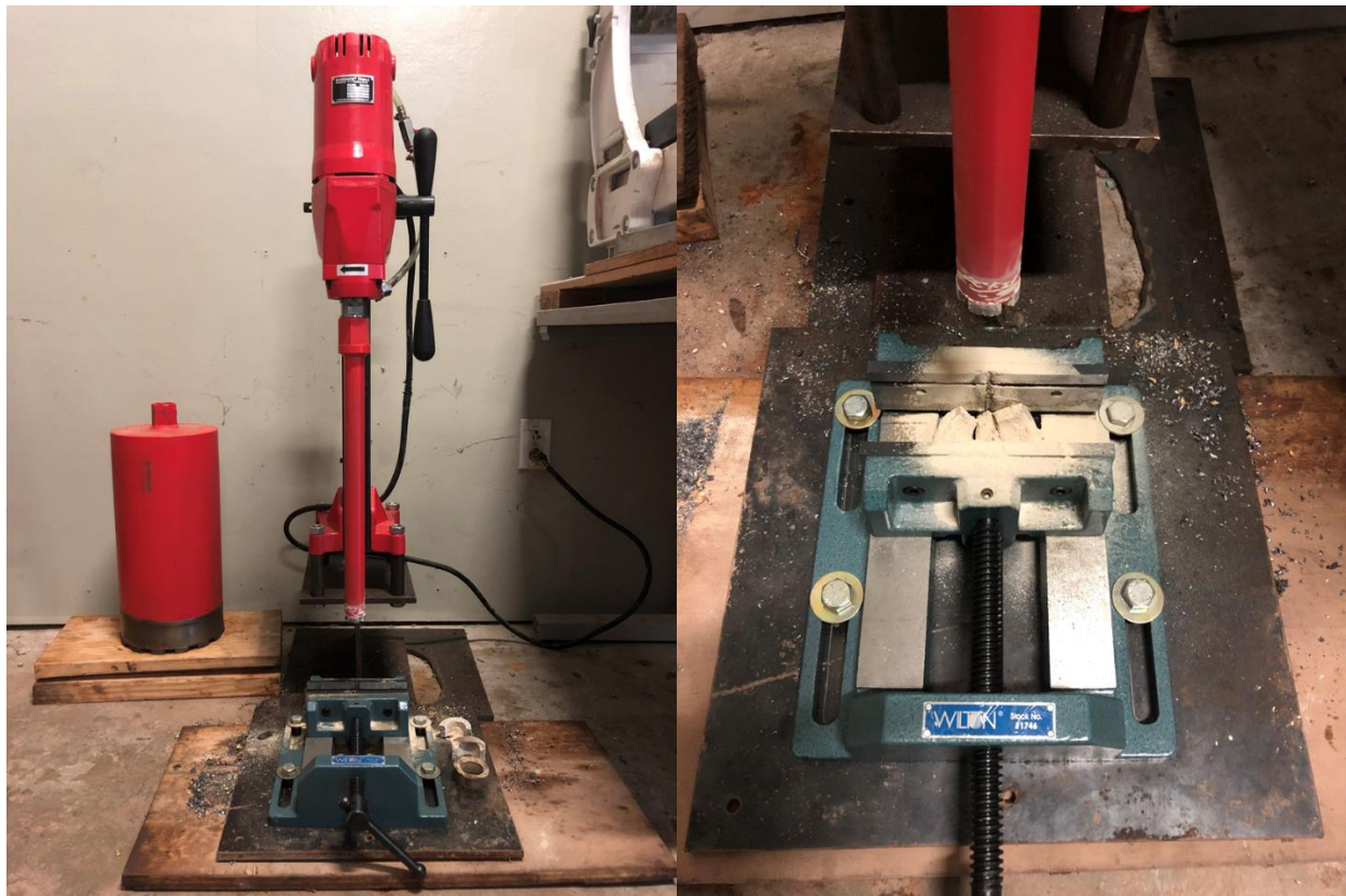
Figure 3. 1. Core Cutting Machine in LSU PETE E-lab Used to Cut Core Plugs and Samples
