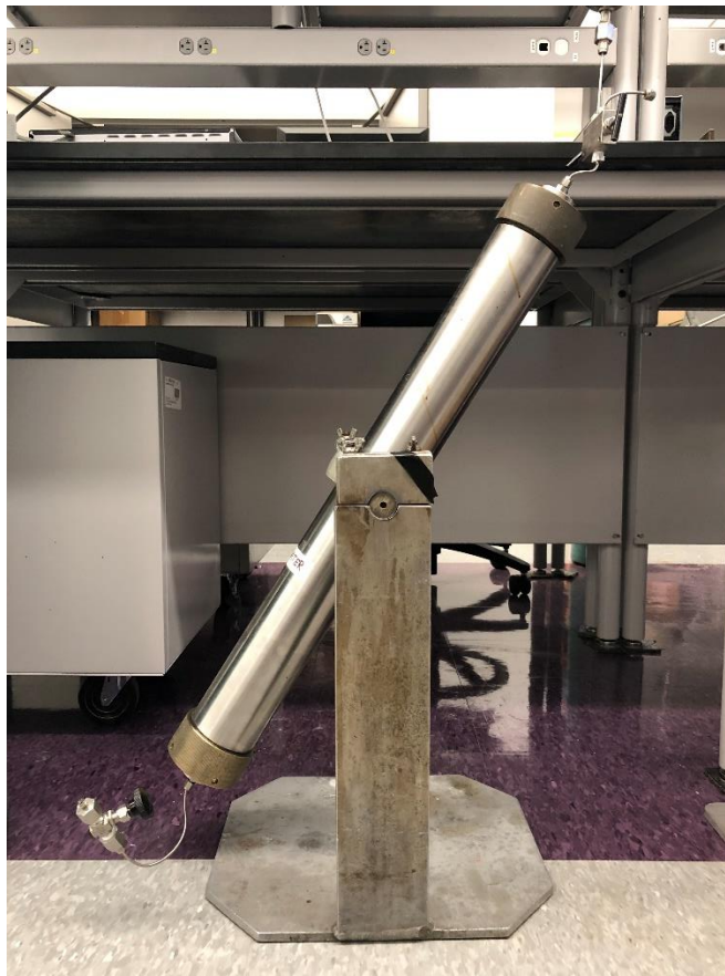
Figure 3. 14. A 2,000 mL Capacity Gas Injection Transfer Vessel Used to Inject Gases into the Cores in EOR Experiments
