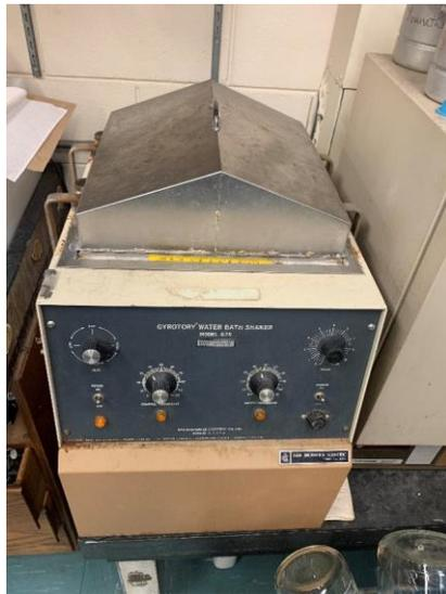
Figure 8. Water bath shaker used to culture 100 mL inoculum.
