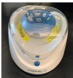
Figure 11. VWR microfuge used to pellet culture samples.
