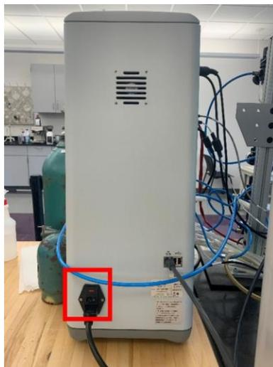
Figure A2. BioFlo 120 power switch.
