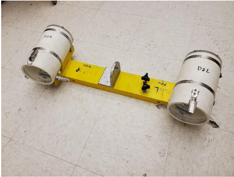
Figure 2. SeaGIS stereo camera housing.
