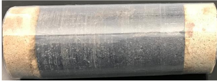
Figure 3.16. The TMS core was fixed tight in a heat shrinkage tube with two Berea sandstone cores placed at each end for pressure support
