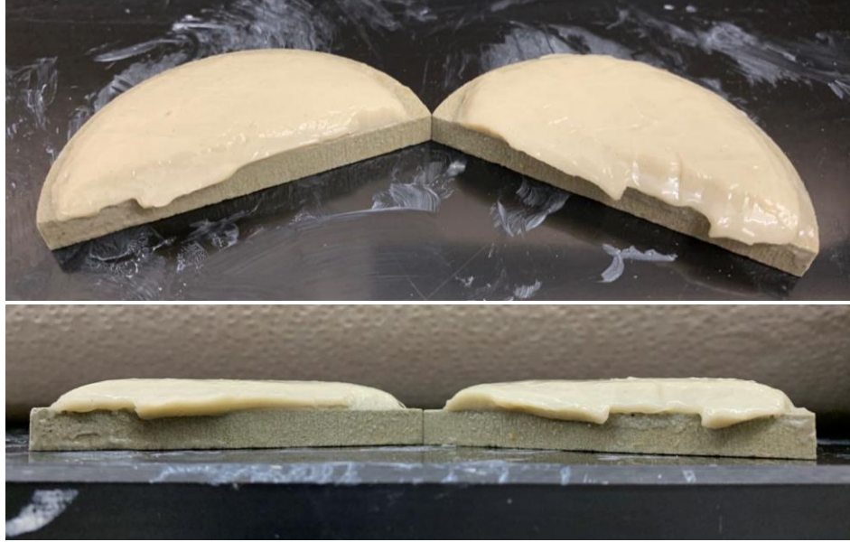
Figure 4.13. Ruptured filtercake (without LCMs) after testing.
