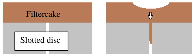
Figure 3.1. Illustration of filtercake rupture in the experiment: filtercake being pushed through a slot and lost its integrity when sustaining high differential pressure, modified after (Cook et al., 2016)
