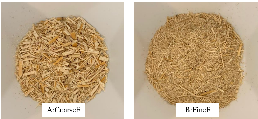
Figure 6.4. Coarse and fine LCMs for plug soaking tests and model calculation: (A) OKCG, denoted by CoarseF; (B) GMF, denoted by FineF.
