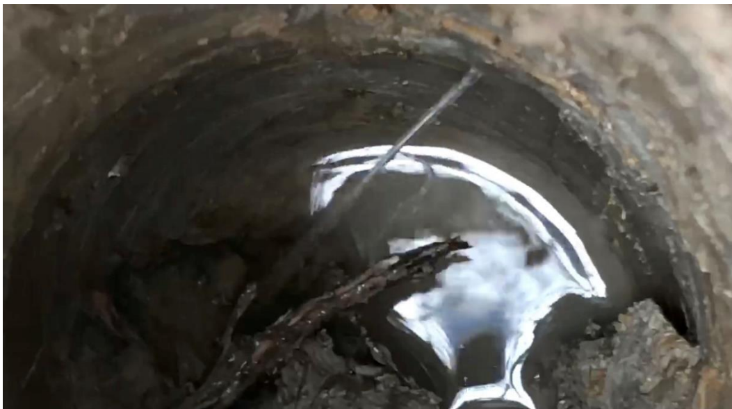
Figure A4. Image of free water flowing from a root channel at the swale site that was intercepted when digging a borehole for soil collection.
