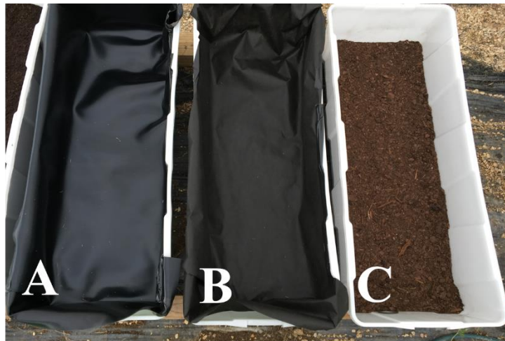
Figure 14. Simulated raised bed barriers applied to containers. Contaminated media sealed by selected barriers up to the top of each container's edge (A. neoprene rubber; B. landscape fabric; C. no-barrier control).
