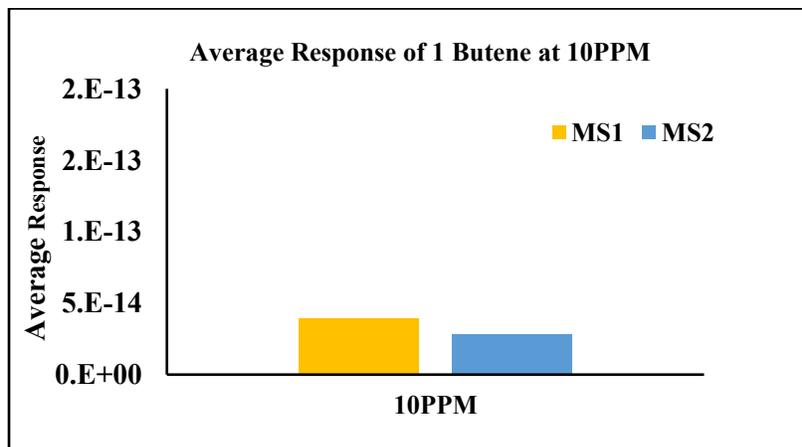
Figure 6. 13. Average Mass Spectrometer Response to 1, Butene
