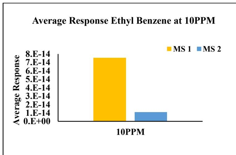
Figure 6. 18. Average Mass Spectrometer Response to Ethyl- Benzene
