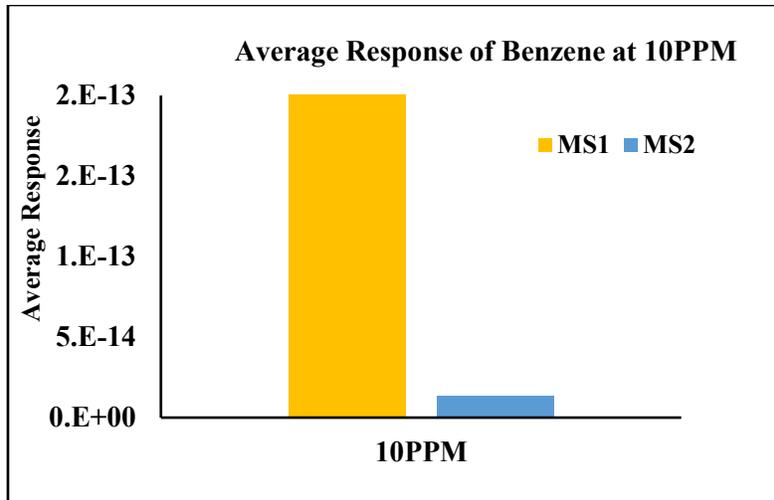
Figure 6. 14. Average Mass Spectrometer Response to Benzene
