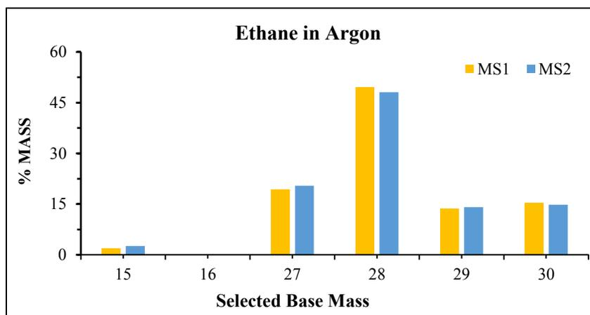
Figure 5. 3. Spectrum of Ethane balanced in Argon
