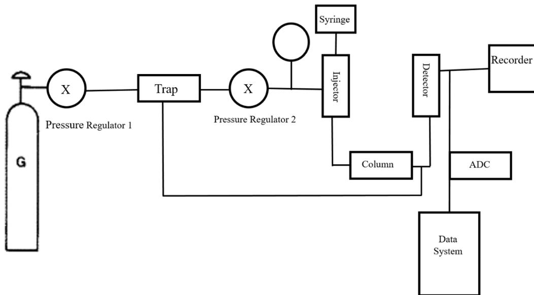
Figure 2. 5. Gas Chromatogram Adapted after Bartle et al. 2002
