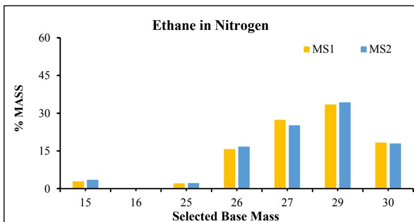
Figure 5. 2. Spectrum of Ethane balanced in Nitrogen
