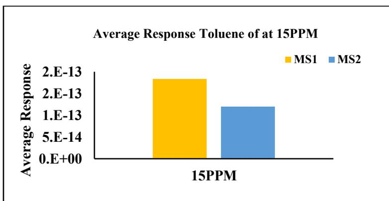
Figure 6. 25. Average Mass Spectrometer Response to Toluene
