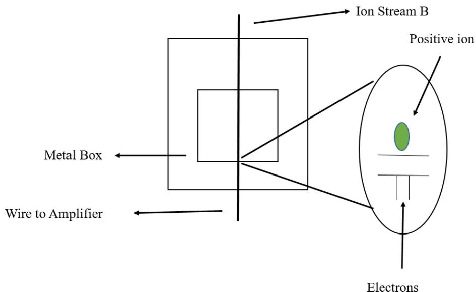
Figure 2. 13. Detector Modified after Clark 2000
