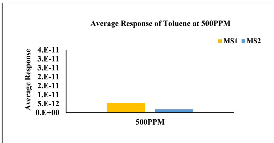
Figure 6. 38. Average Mass Spectrometer Response to Toluene
