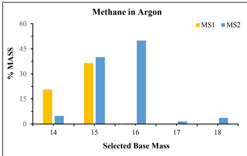
Figure 5. 1. Spectra of Methane in Argon
