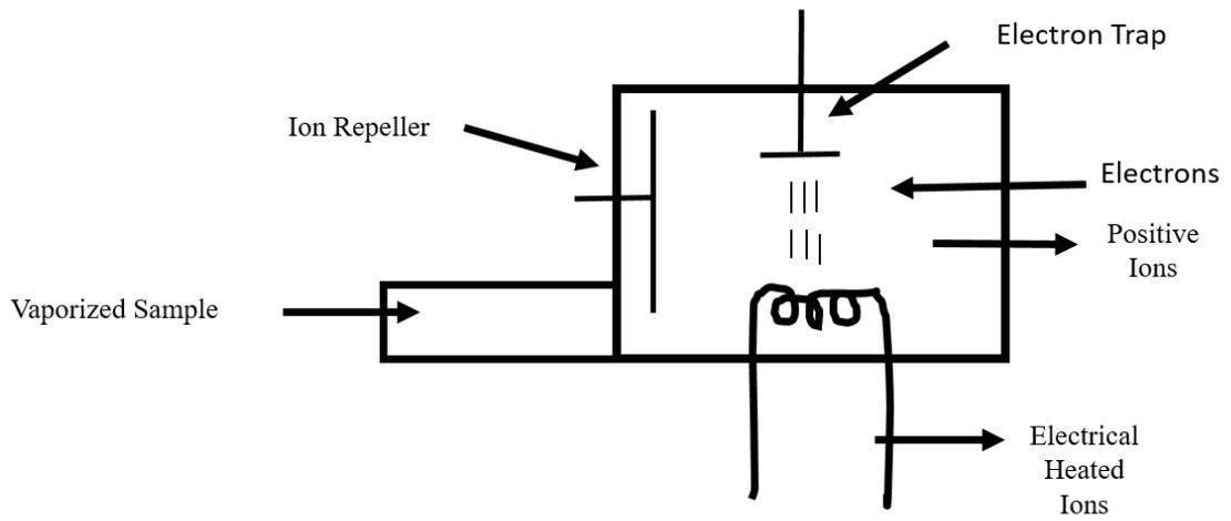
Figure 2. 10. Ionizer Adapted from Clark 2000
