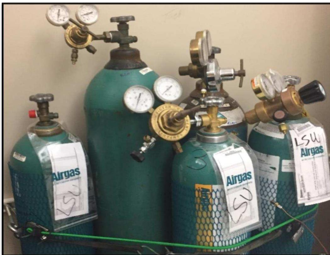
Figure 4. 4. Mixed Standard Cylinder used in Experiment
