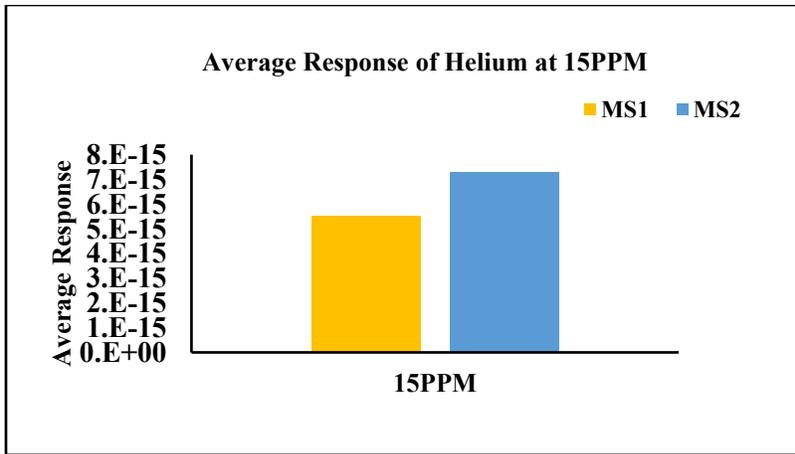
Figure 6. 21. Average Mass Spectrometer Response to Helium
