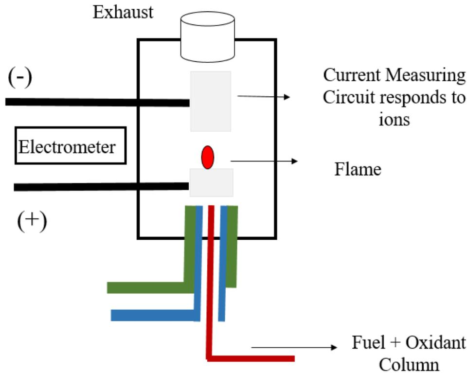
Figure 2. 6. Flame Ionization Detector (FID) Modified after Chaulya et al., 2016
