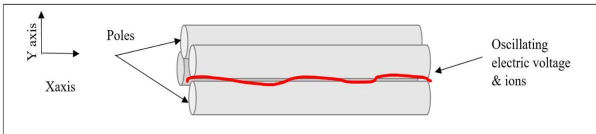
Figure 4. 3. Schematic Picture of a Quadrupole Mass Analyzer
