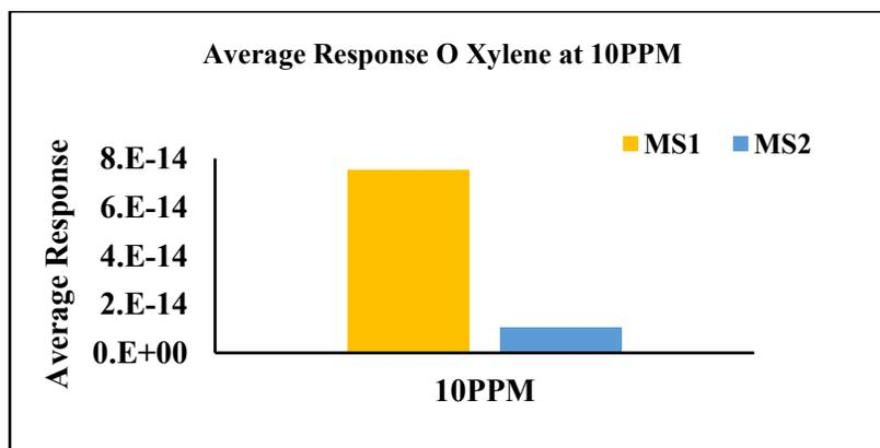
Figure 6. 16. Average Mass Spectrometer Response to O Xylene
