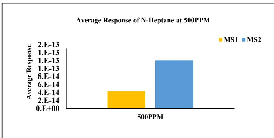
Figure 6. 39. Average Mass Spectrometer Response to N- Heptane
