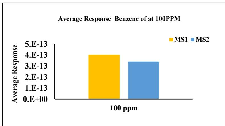
Figure 6. 30. Average Mass Spectrometer Response to Benzene
