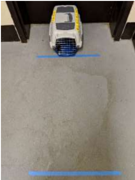
Figure 2.5. Experimental set-up for collection of exposure rate data. The distance between the blue tape is 100 \pm 1 cm.
