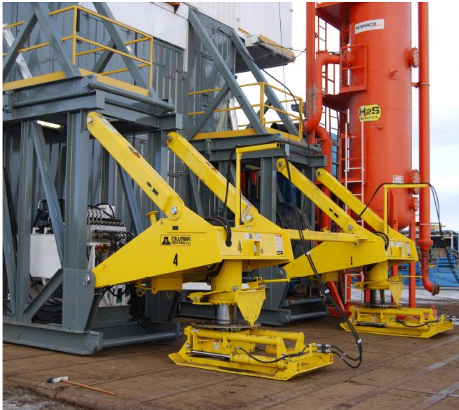
Figure 2.2. An Example of the Rig Walking System, From Columbia Industries
