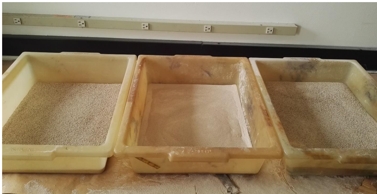
Figure 5. Zeolite particle size classification. Left to right: unclassified or higher than 710 microns, below 355 microns, optimal size between 355-710 microns.
