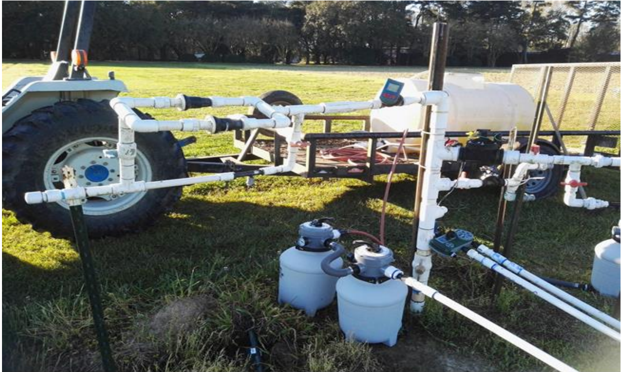
Figure 7. Zeolite filtration arrangement. Tank with inoculated water, pool filtration system with sand zeolite.
