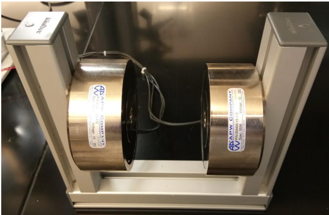
Fig. 8. Flat-faced round holding solenoid electromagnet
