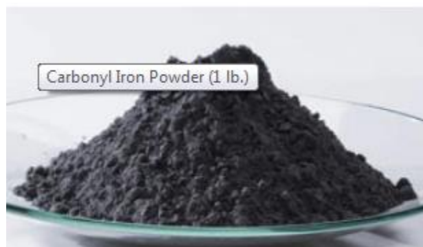
Fig. 6. Carbonyl Iron Powder in dry state
