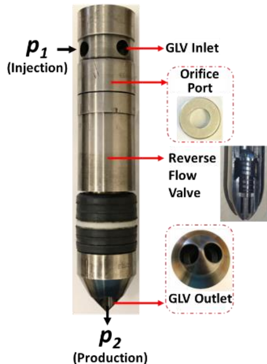
Figure 2.8. Orifice GLV geometry [ adapted from Coutinho (2018)].
