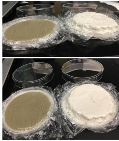
Figure 8.2. Filter cake generated by low gravity solids drilling mud without HGS (sample at left), and with a high concentration of HGS (right).
