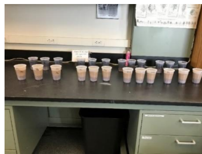
Figure 2.1. Flooding of substrates treated with four termiticides in cups
