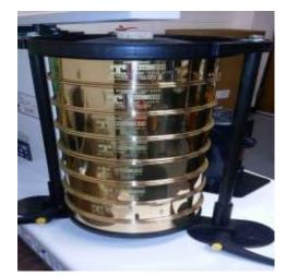
Figure 0.5. Mechanical Sieve shaker used to separate the crushed carbonate rocks into different sized particles.
