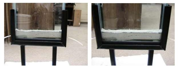
Figure 0.9. Placement of a 2" layer of higher sized carbonate grains (600 µm) in the model
