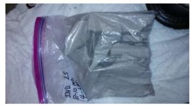
Figure 0.3. Chunks of Indiana Limestone rock as received from the supplier
