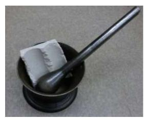
Figure 0.4. Crushing of the rocks using a mortar and pestle
