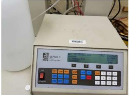
Figure 3.2. Pump Controls for the Series D Pump
