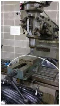
Figure 0.6. Drilling machine used to drill holes in the pipe used as a horizontal well for the experiments.
