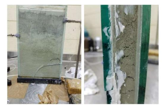
Figure 3.4. Cracked model due to the increased pressure
