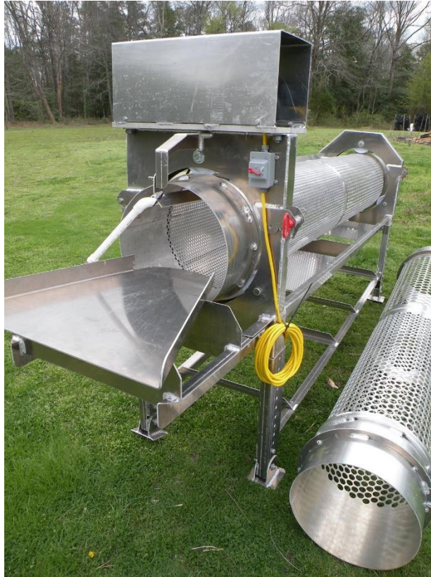
Figure 6.4. QuickTube Sorter manufactured by the Chesapeake Bay Oyster Company, available for use by local growers at the Louisiana Sea Grant Oyster Research Laboratory, Grand Isle, LA. Sorter consists of interchangeable rotating tubes with various hole sizes to sort seed and larger oysters. Oysters are pushed down the sloping rotating tube by water jets.
