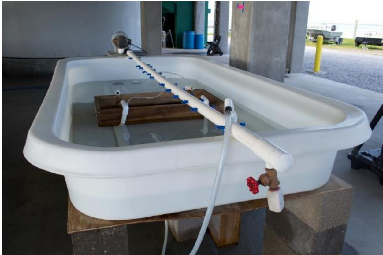
Figure 5.13. Setting tank. A blower is connected to a manifold that runs along the length of the tank. Flexible rubber tubing connects the manifold to the airlifts attached to setting trays. Water is recirculated from a reservoir by a sump and discharged through a hose positioned at the end opposite the stand-pipe.
