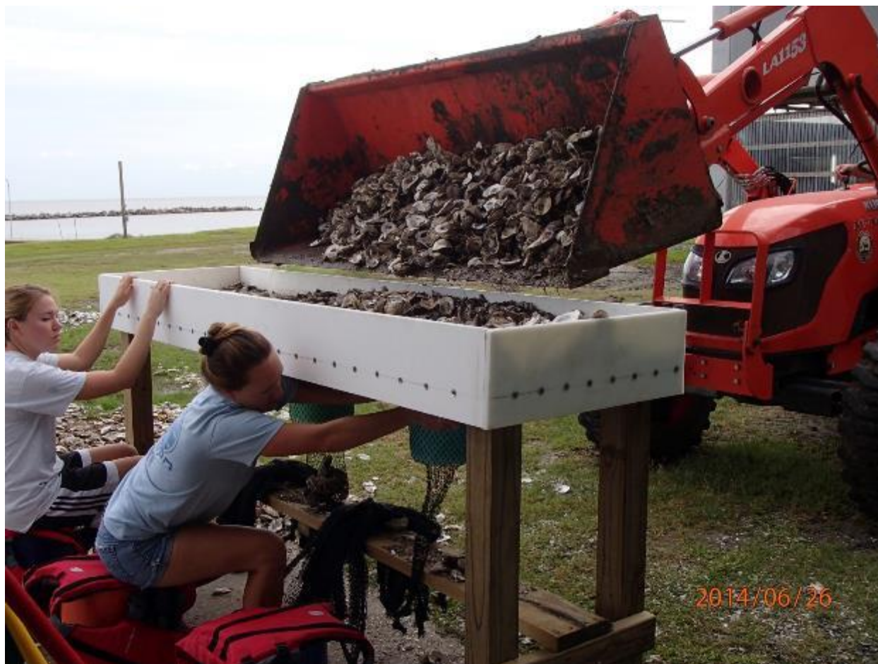
Figure 5.9. Shell bags being filled at a table designed to aid in filling. Bags are slipped over the PVC pipe affixed to the table; cultch is then loaded onto the top of the table and pushed into the openings filling the bags.
