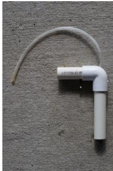
Figure 5.16. An airlift. 'L' shaped airlift with flexible air-hose and air-stone (top left). The air-hose is inserted into the airlift through a hole in the elbow and the air-stone attached to the hose (top right). The air-stone has to be pulled up into the airlift for water to be lifted (bottom).
