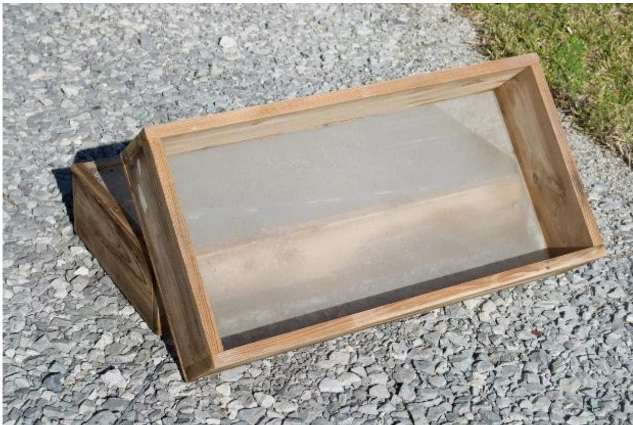
Figure 5.15. Wooden (cypress) setting tray with mesh bottom (measuring 32" x 16" x 6").
