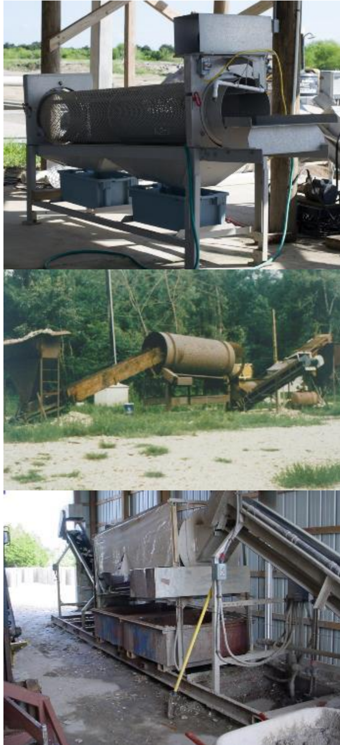
Figure 5.10. Oyster size graders that can be used to grade and wash seed simultaneously. Seed oysters or cultch materials are loaded into the grader as the drum rotates and water is sprayed into the rotating drum washing shells and allowing oysters/shells to fall through appropriate sized holes in the drum for grading.
