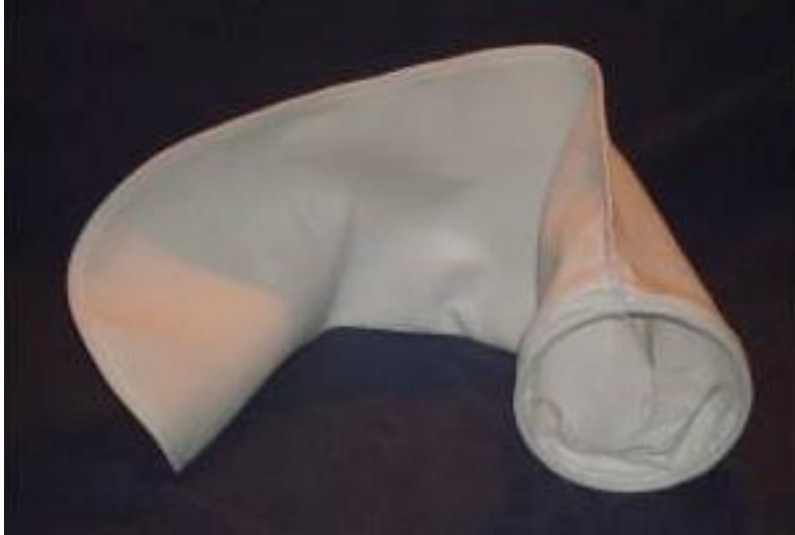
Figure 5.7. Filter bag that fits over the setting tank source of seawater.
