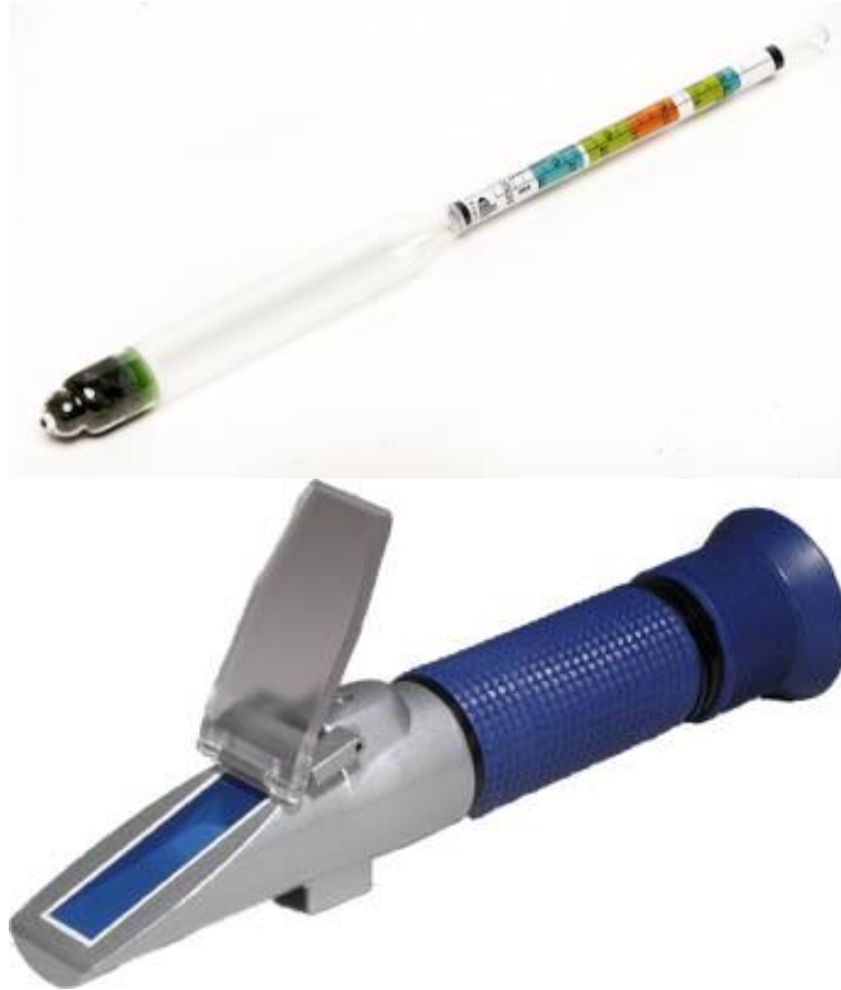
Figure 5.2. Tools with which salinity (salt content) may be estimated: hydrometer (top) and refractometer (bottom).
