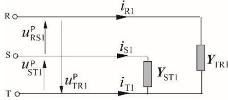
Figure 7: Specific structure of equivalent circuit of the arc furnace for the fundamental harmonic with
