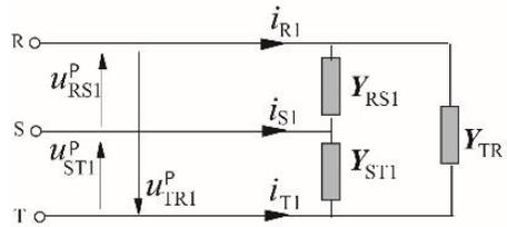
Figure 6: General structure of equivalent circuit of the arc furnace for the fundamental harmonic
