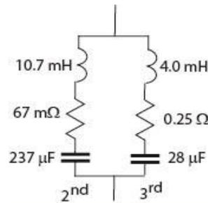
Figure 24: Structure and parameters of a filter of the 2<sup>nd</sup> and the 3<sup>rd</sup> order harmonics
