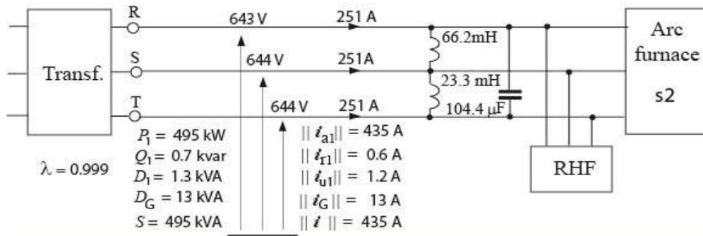
Figure 27: The results of balancing a furnace in the state s2 with a RHF of the 2<sup>nd</sup> and the 3<sup>rd</sup> harmonic
