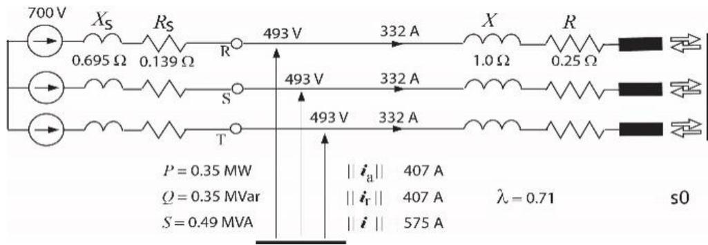
Figure 3: The results of modeling of a furnace which operates
