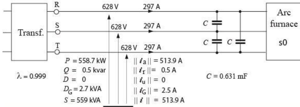
Figure 12: The results of modeling of reference furnace in state  $s_0$
