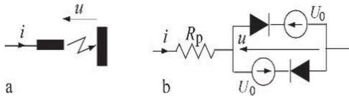
Figure 2: A circuit (b) that approximates the arc (a).
