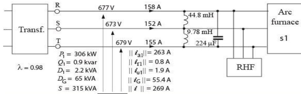
Figure 25: The results of balancing a furnace in the state s1 with a RHF of the 2<sup>nd</sup> and the 3<sup>rd</sup> harmonic
