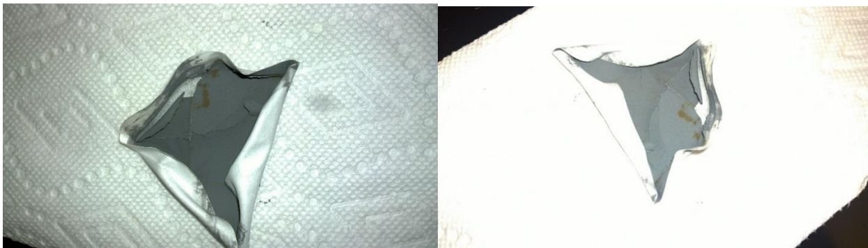
Images of Sample 2 filter paper at 5 days (left) and 7 days (right) after filter press test.
