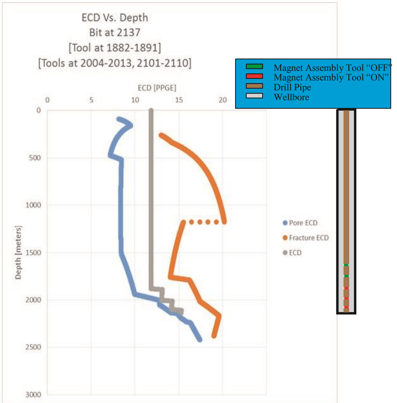
ECD with Pore pressure ECD and Fracture pressure ECD with bit at 2137 and fourth magnetic assembly tool not applying a magnetic field.
