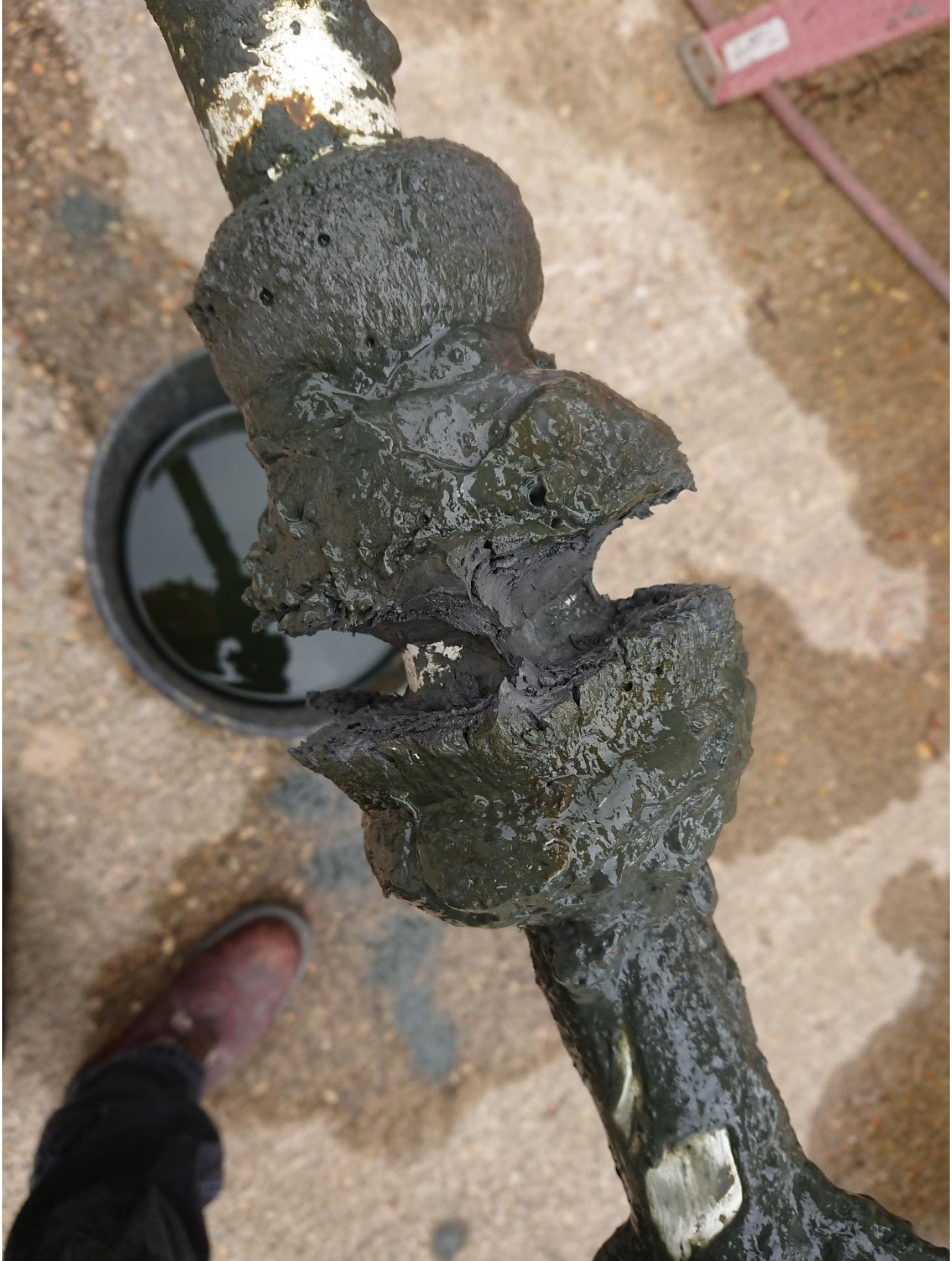
Image of gelled particles around magnets after a large amount had been physically removed
