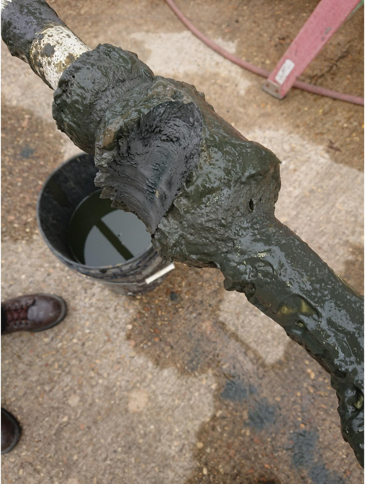
Image of gelled particles around magnets after a portion had been physically removed
