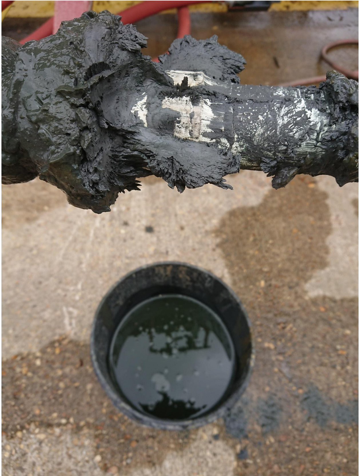
Image showing gelled fluid aligned with magnetic field lines
