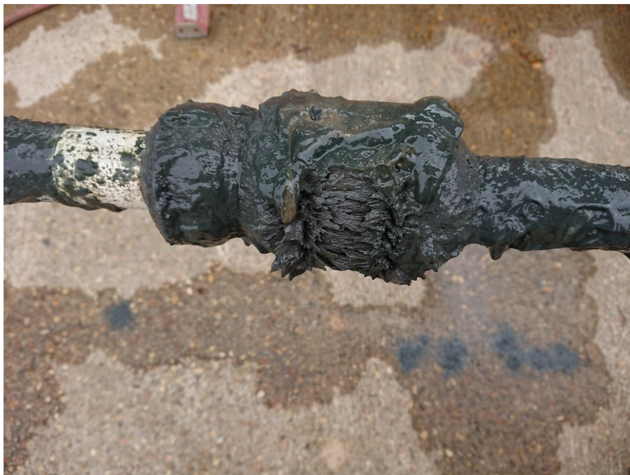
Image of gelled particles around magnets showing magnetic field lines
