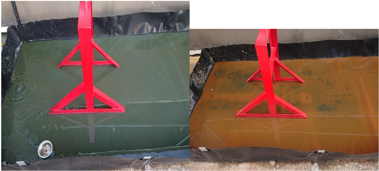
Images of fluid during (left) and 2 days after (right) cleaning.
