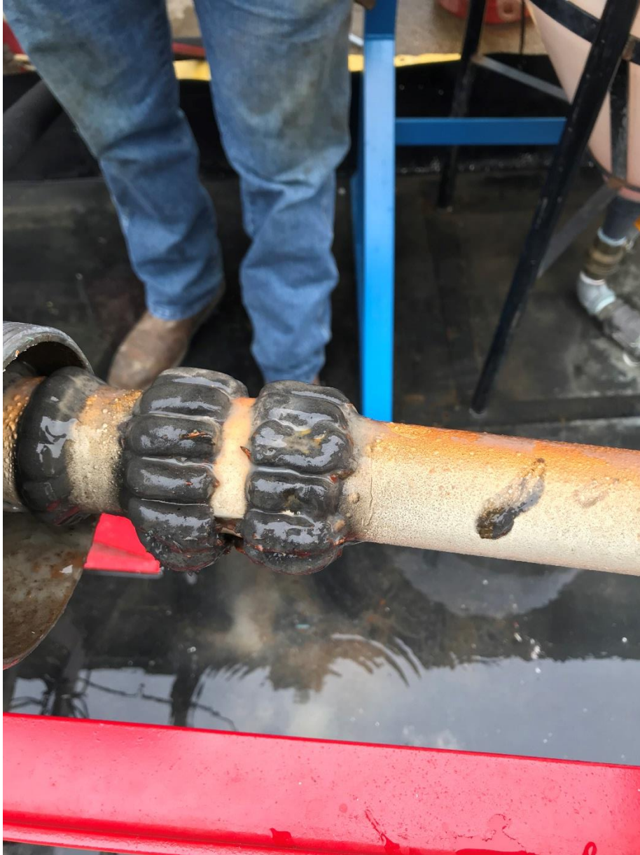
Image of particles built up around magnet rings after barite experiments.
