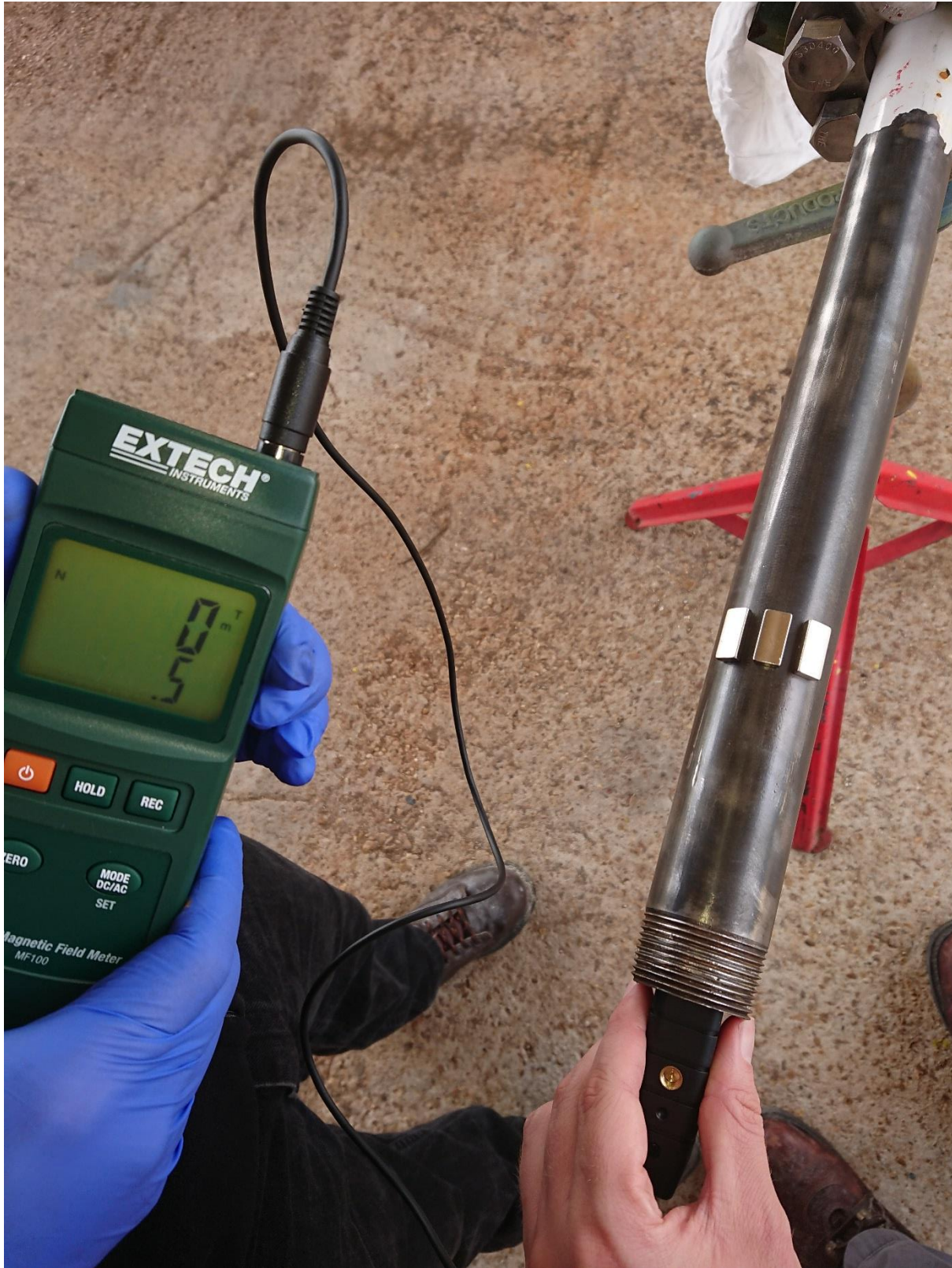
Image showing a 0 Gauss reading with the probe placed against the inside of the inner pipe next to the magnets.
