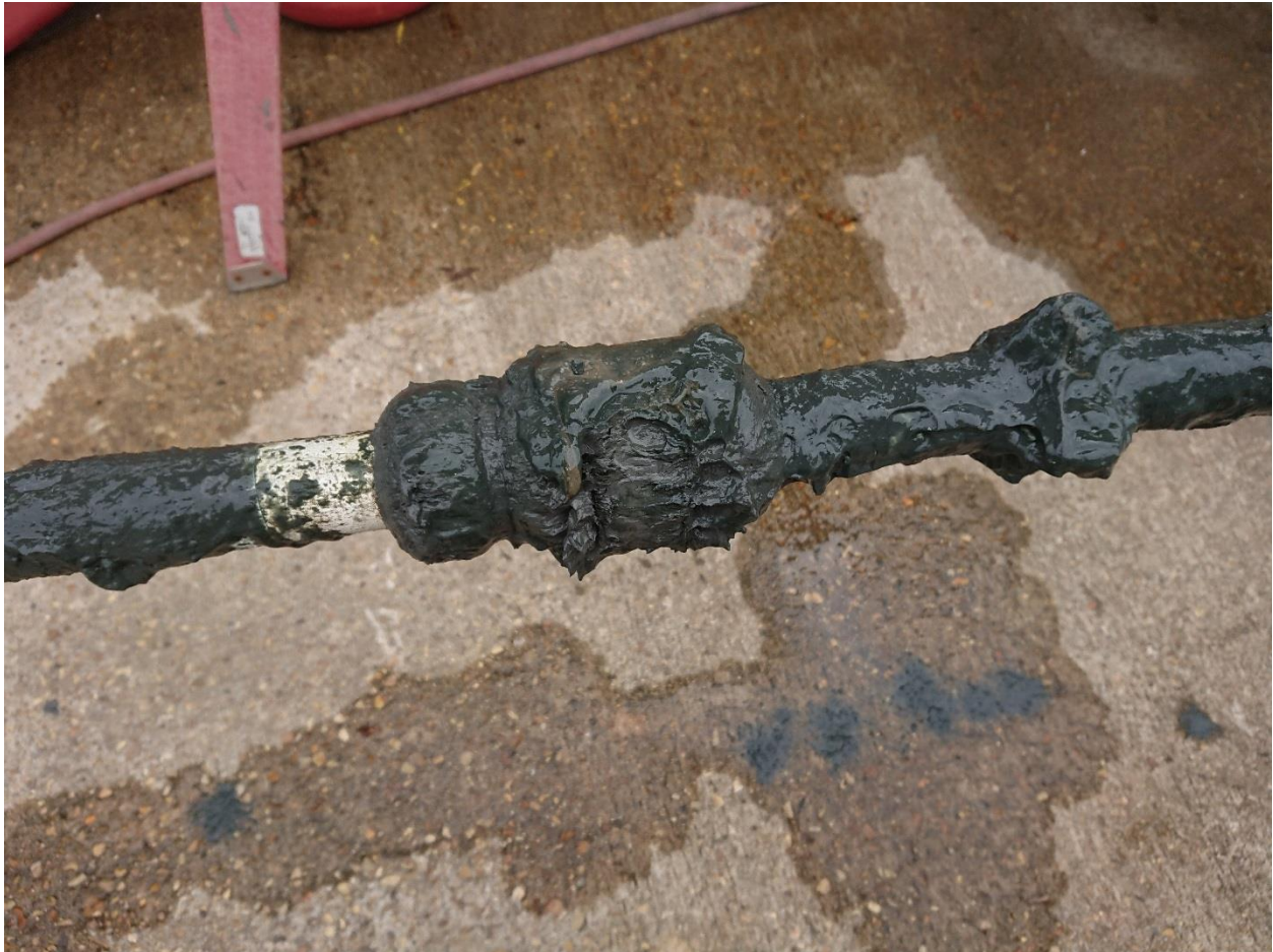
Image of particles built up around magnet rings after magnetorheological experiments.
