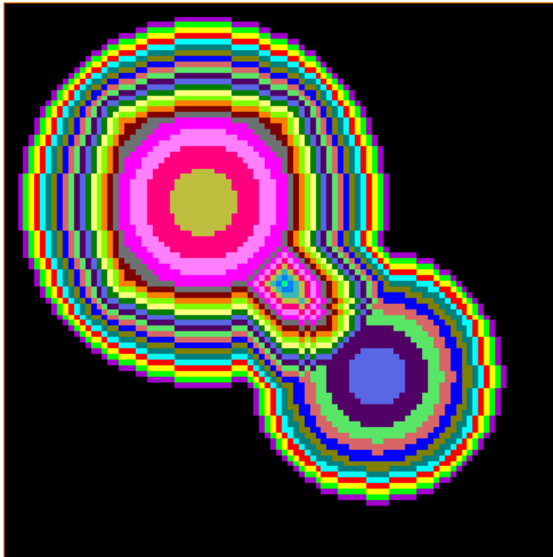
Figure 3.14. Burn map for two overlapping spheres, 100 voxels per side with a nominal voxel width of 0.01 cm
