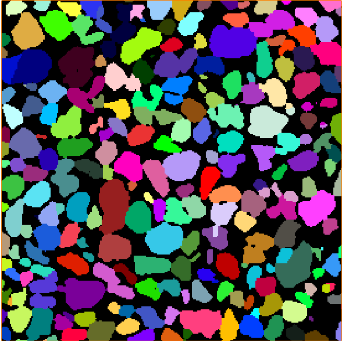
Figure A.8. Ottawa sand 7 after trial 2 logistic regression equation, 2993 grains, 3.025 mm per side, 275^3 voxels
