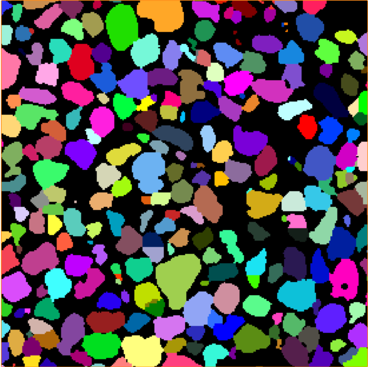
Figure A.10. Ottawa sand 10 VOX2GRAINS updated output, 3960 grains, 3.025 mm per side, 275^3 voxels
