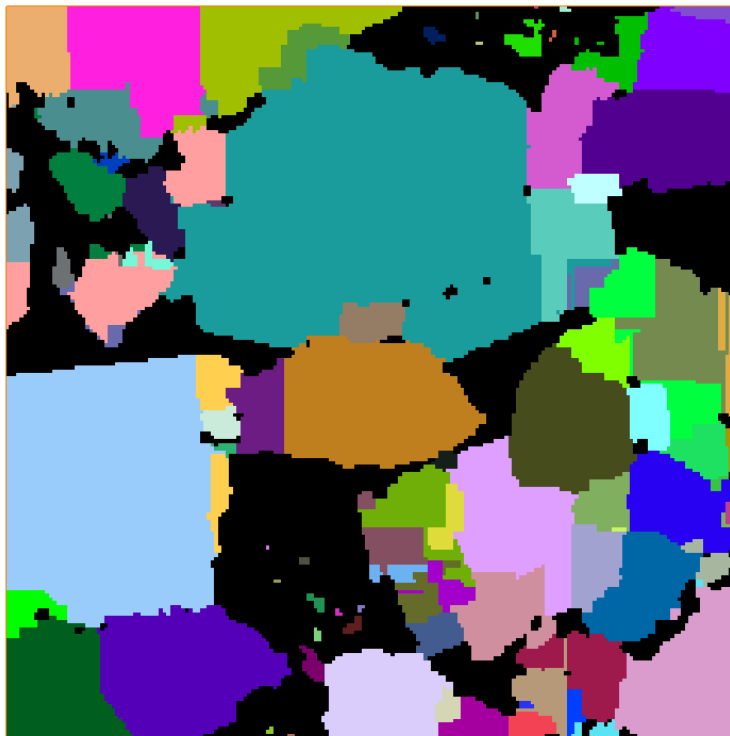
Figure 3.4. Partitioned image of quartz-feldspar rock using connectivity values of six, 820 \mu m per side, 200 3 voxels
