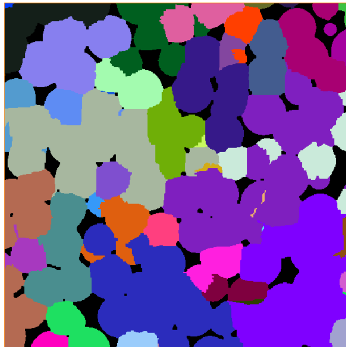
Figure 3.16. Refined output using the initial automerger logic with a contact area to surface area ratio of 0.15, 500 voxels per side with a nominal voxel width of 0.01 cm/voxel
