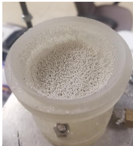
Figure 13: Static Cling Observed by Porcelain Particles
