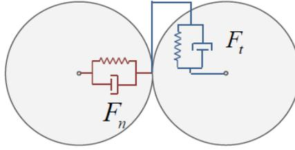
FIGURE 4.3. Linear spring dashpot model assumed for DEM, including a dissipative viscous dashpot at the contact point to account for energy dissipation due to plastic deformation
