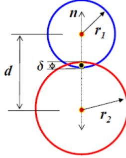
FIGURE 4.2. Overlap between particles, representing the deformation given by  $\delta$
