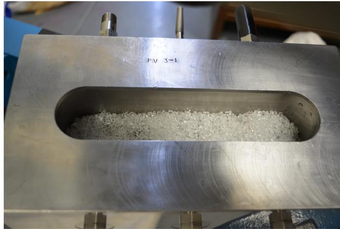
FIGURE 3.1. Conductivity cell loaded with smart proppants
