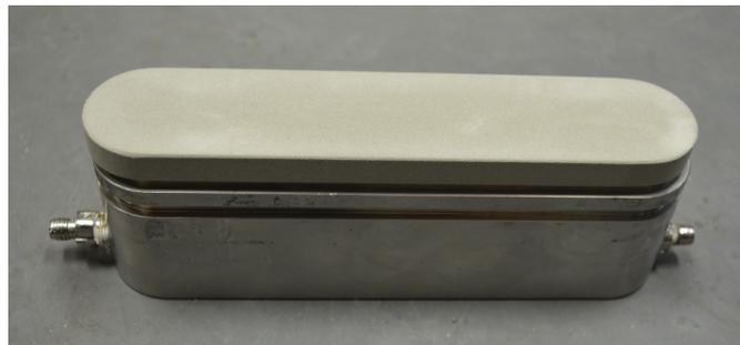
FIGURE 3.2. Side piston and sandstone conductivity core
