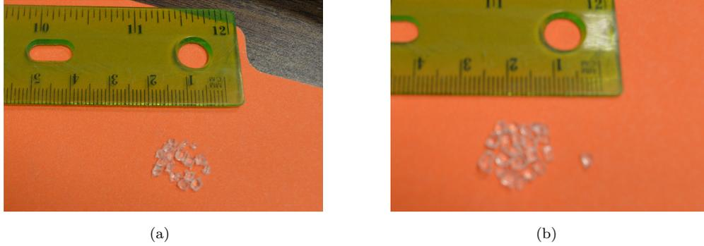
FIGURE 2.3. Smart proppants a)Before activation; b)after activation
