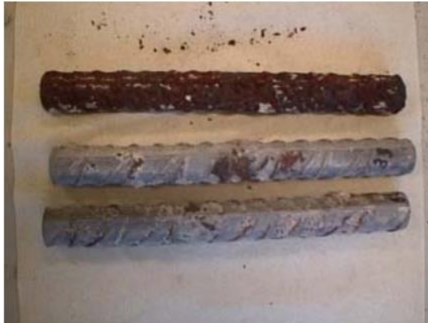
Figure 2.16 Rebar Removed from Cylinders with 3.2% NaCl (Chlorides) Intermixed after 3 Years of Storage at 38°C and 90% RH. Upper, Middle and Bottom Bars are from Control, 2%CN Admixed and 4%CN Admixed Concrete Respectively (Justnes 2005).
