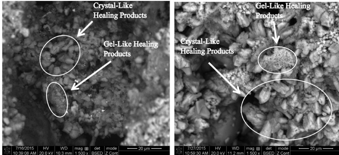
Figure 3.7 Healing Products in Mortar Specimen Crack (Left: 1% Microcapsule Content - Right: Control)
