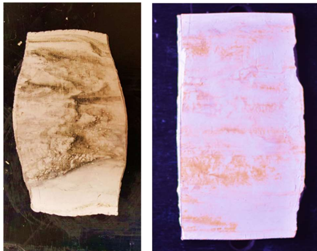
Figure 23: Discoloration due to metal corrosion (left) and over-heating (right).
