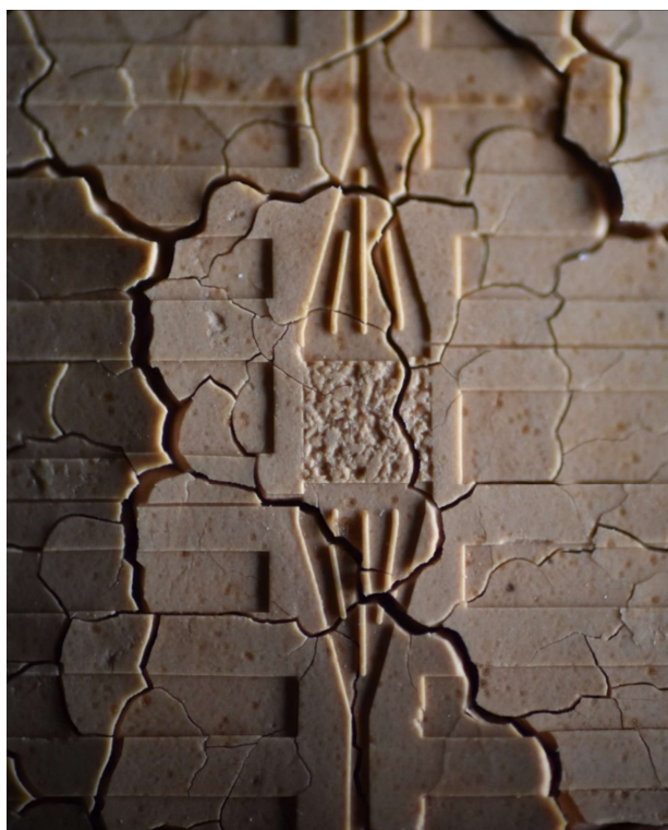
Figure 37: Sintering at 1450°C resulted in warping and cracking of the Berea sample.
