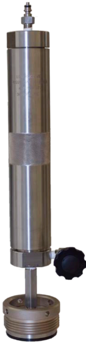
Figure B2- LCM Receiver that gets attached to the PPA cell instead of the backpressure receiver.
