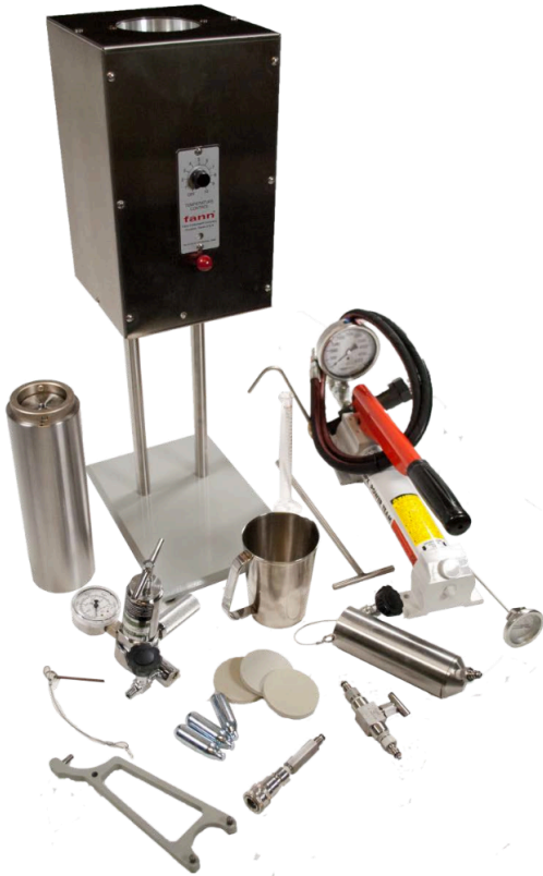
Figure 2.1. High Pressure and High Temperature Permeability Plugging Apparatus
