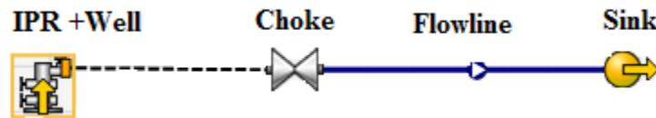
Figure 4.10 Schematic of well with IPR model included
