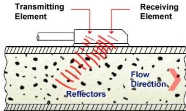
Figure 2.7 Ultrasonic flow meters (Al-Yarubi 2010)
