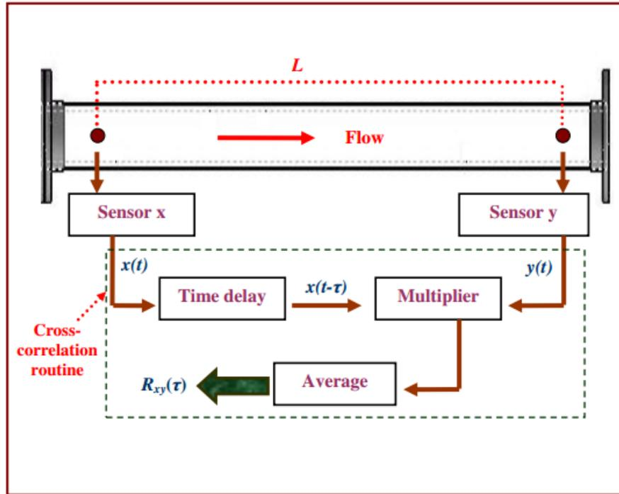
Figure 2.9 Schematic diagram of a cross-correlation flow meter (Hasan 2010)
