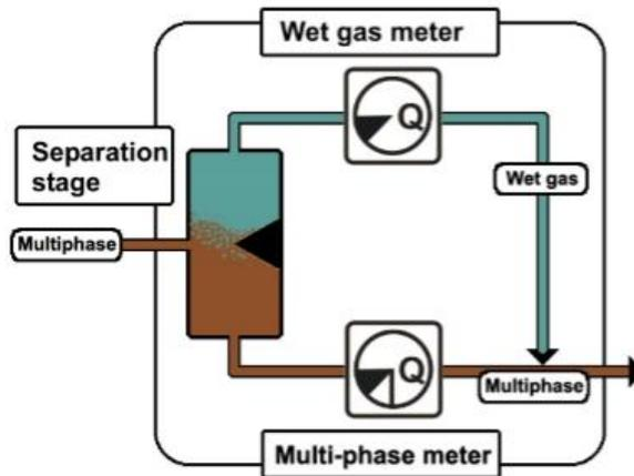
Figure 2.11 Partial separation with two measurement loop (Corneliusen 2005)
