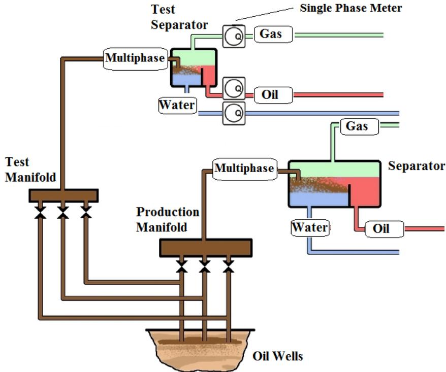
Figure 2.1 Production separator and test separator
