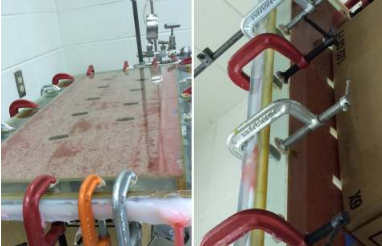
Figure 5.38: Picture of the model early in the progress of the horizontal gas flood (Left): Shows the topside of the model, (Right): Shows the underside of the model contemporaneously with the Top side
