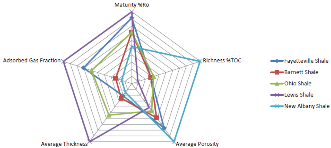
Figure 1.4: Properties of various shale gas reservoirs around the continental United States. Each reservoir is unique in terms of thermal maturity, adsorbed gas fraction, thickness and so on. The reservoir maturity, evaluated by measuring vitrinite reflectance, is a measure of the degree of heating shale has been subjected to. Richness, or percentage total organic carbon is the amount of organic matter in a given sample of rock.
