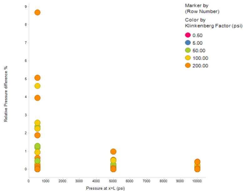
Figure 7.7: Relative pressure change % depends heavily on pressure, the lower the pressure the more pronounced the effect, linear case
