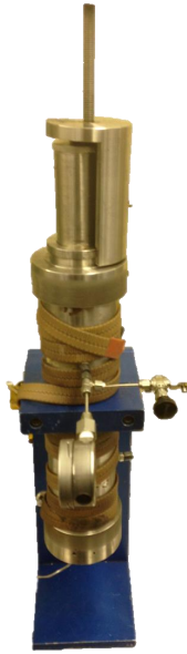
Figure 5.13: Core holder situated vertically for GAGD experiments
