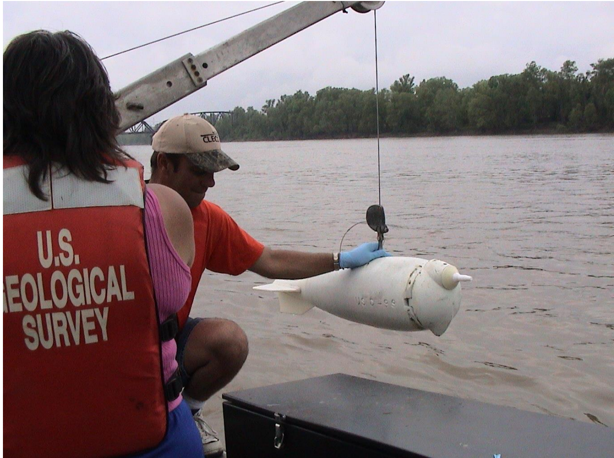
Figure 3.2: An example of depth integrated sampler used by United States Geological Survey (USGS) personnel while sampling suspended sediment concentration (SSC in mg/l) in the Atchafalaya River. The same samplers are used to sample SSC in the Lowermost Mississippi River. Picture courtesy: Dr. Y. Jun Xu.
