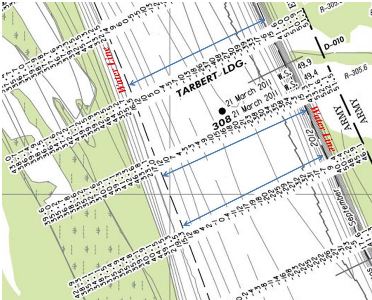
Figure 2.2: Screen-shot kept from the LmMR Hydrographic Survey Book of 2013 (USACE, 2013) showing schematics of three cross-sections at Tarbert Landing. ‘Water Lines’ in red represent the black dashed water surface lines marked by USACE denoting the top bank elevations for both ends of the cross-section. The elevations of the cross-sections measured are shown next to the blue line. All the elevations on the Hydrographic Survey Book are in feet and have been converted to meters for channel analysis in this study.
