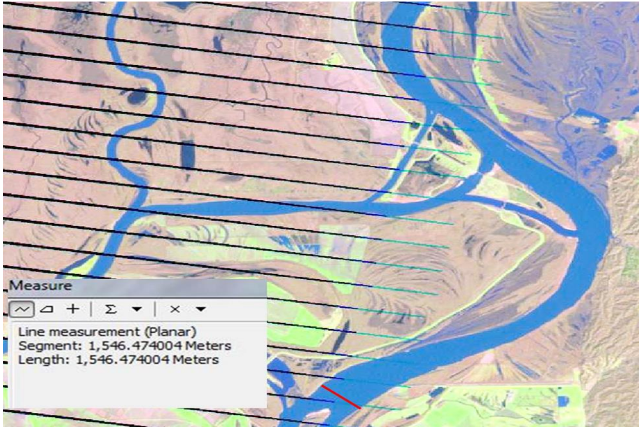
Figure 4.2: Screenshot of the Landsat 7 Satellite image for Tarbert Landing of the Lowermost Mississippi River. The image was collected in .tiff format using the USGS Earth Explorer tool. The red horizontal line represents the river width of the LmMR at Tarbert Landing on the date of imagery. The image was directly opened in Arc Map 10.2 and then the river width was measured using the ‘Measure’ tool. The same procedure was followed for measuring river width at Tarbert Landing, St Francisville and Baton Rouge for, respectively, 55, 37 and 42 days during 2004-2015.
