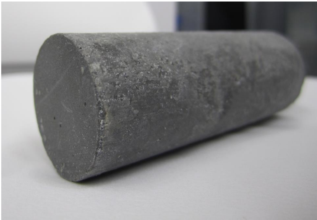
Figure 3.3: Visual sample design of composite core made of kaolinite, cement and polymer PEEK micro-tubes which are not evenly distributed as envisage through SolidWorks©.
