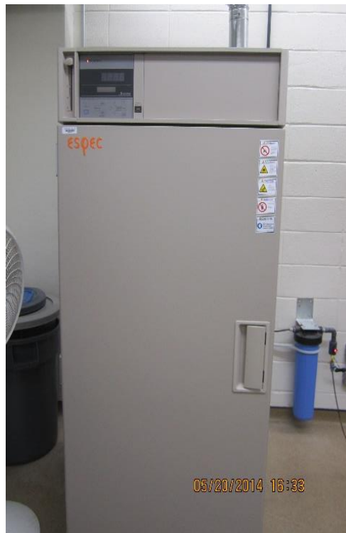
Figure A.4: Automated oven for temperature control
