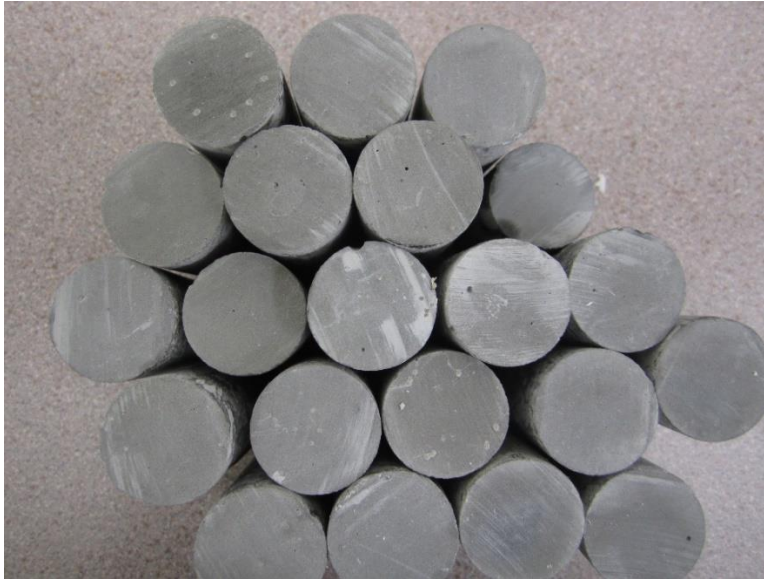
Figure 3.4: Multiple samples of composite core made of kaolinite, cement and polymer PEEK micro-tubes to mimic fractures.
