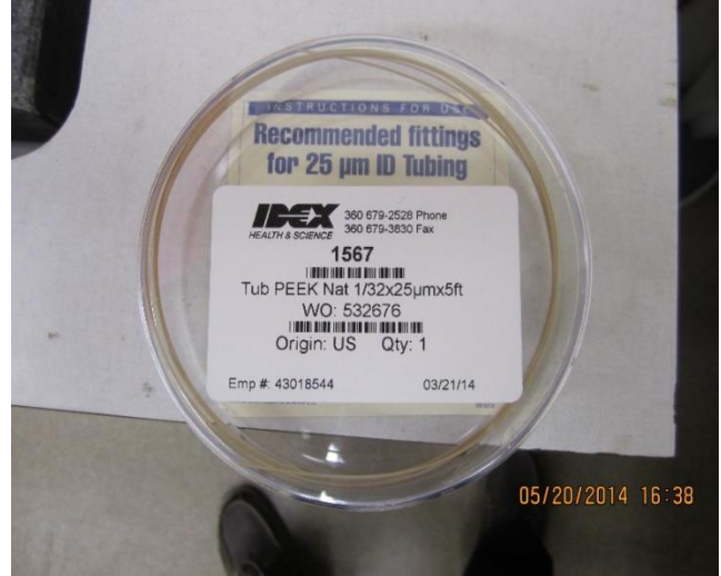
Figure A.6: PEEK micro-tubing used in composite
