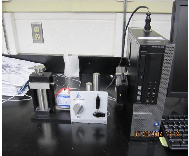
Figure A.2: Helium porosimetry unit for estimation of porosity of fractured cores
