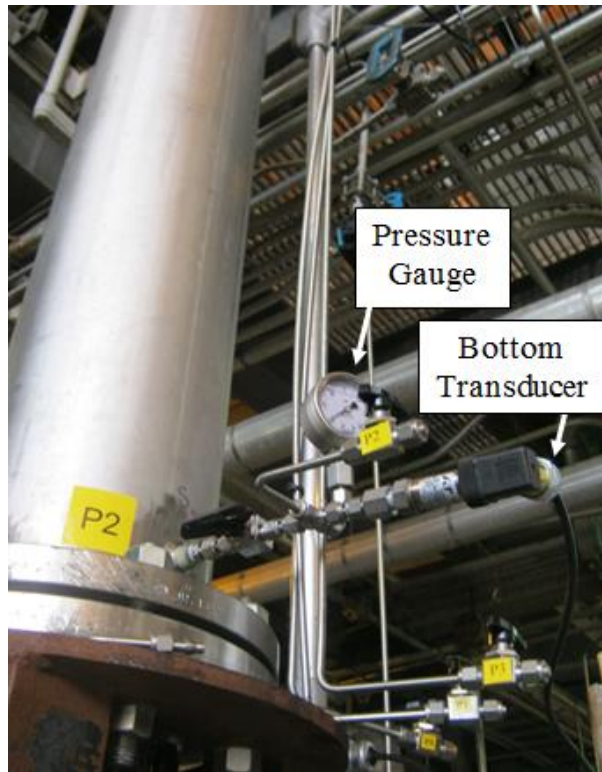
Figure 5.2: Bottom of outer casing with pressure instruments
