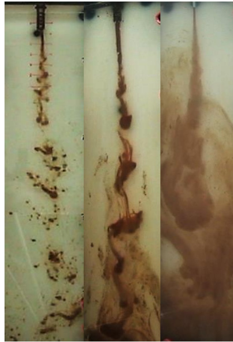
Figure 4.27: Rayleigh mechanism (left), transition (middle) and atomization modes (left) from experiments #20, #42 and #44 respectively
