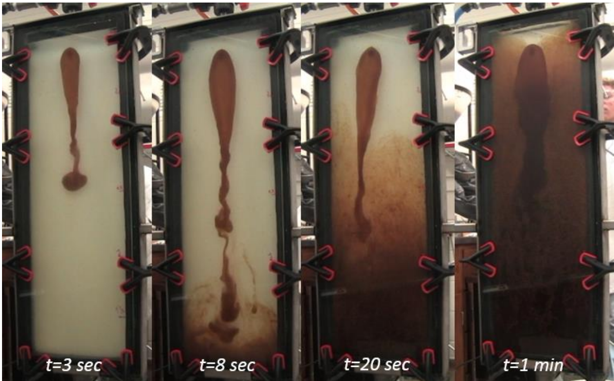
Figure 4.22: Side injection of KF1701 into TF0107 at 2 gpm (Experiment #34). Higher flow rate creates a blurry interface between fluids.
