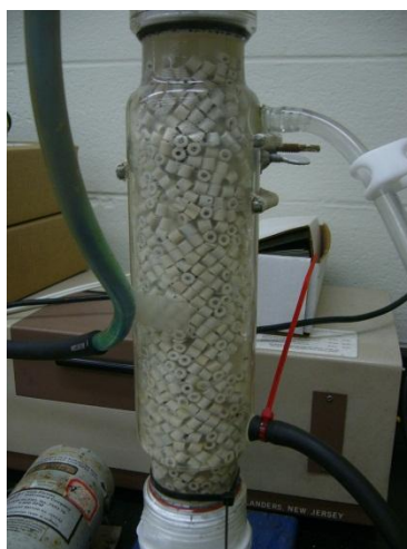
Figure 6 Immobilized cell column filled with ceramic Raschig rings
