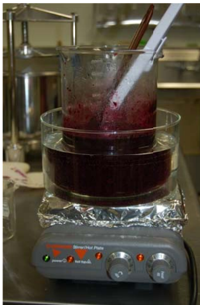
Supplemental Image A.2 Bench top juice experiment water bath used for heating blueberries to 95°C.
