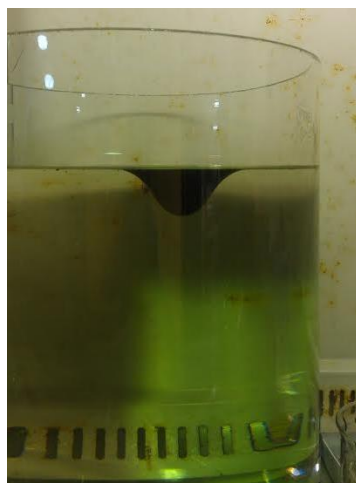
Figure 1-B. Slick sags down after lighter volatile components evaporate
