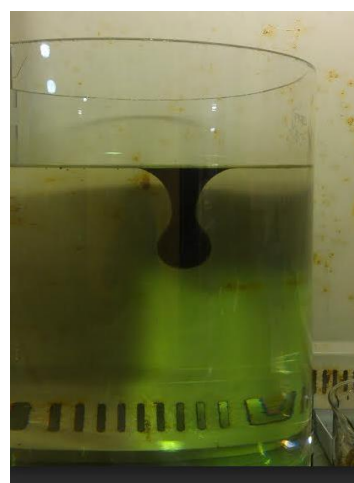
Figure 1-C. Droplet breaks off from slick and falls to bottom of jar.
