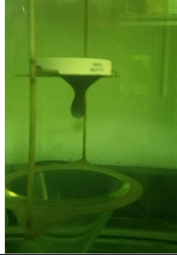
Figure 6: Psuedo-component crude oil droplet about to sink into cone shaped vessel due to dissolution
