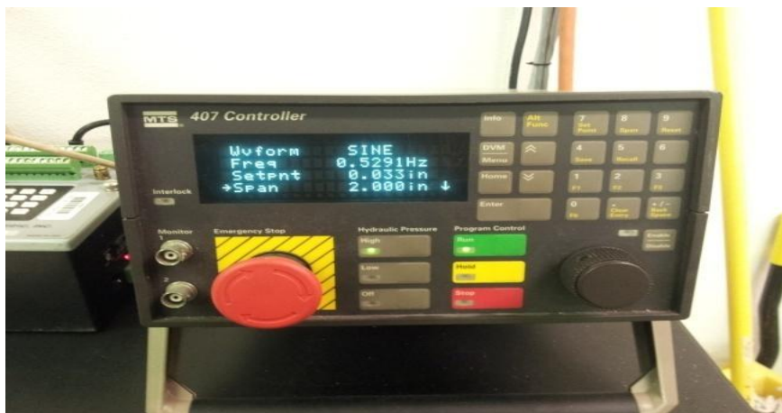
Figure 19 MTS 407 Wave Tank Controller set to Wave Type I , .53 hz, 2” span
