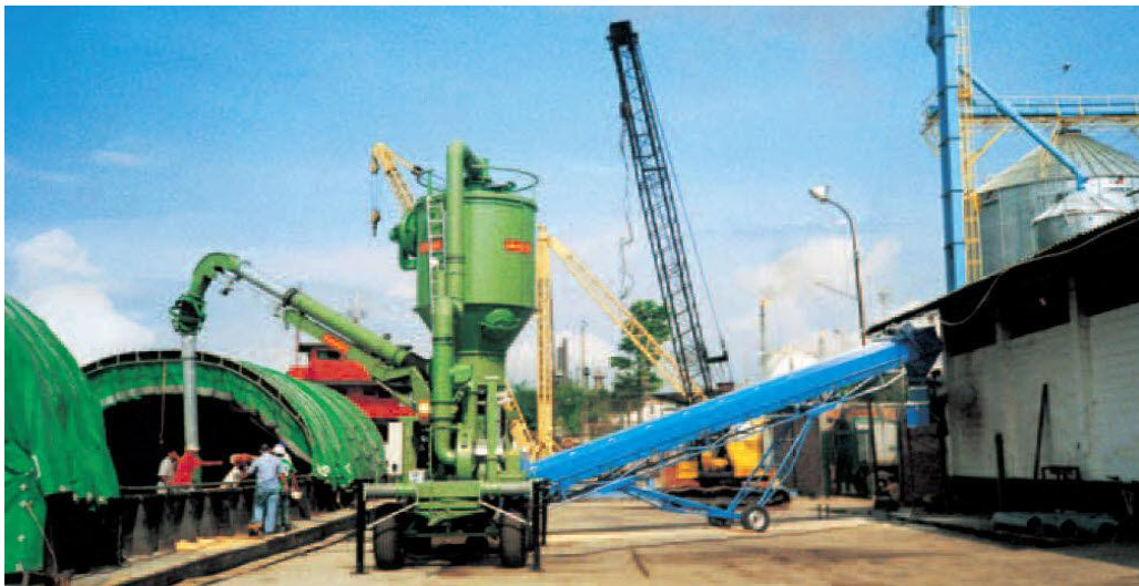
Figure 29 A pneumatic bulk loader loading from a barge at a port facility (Neuro, 2013)
