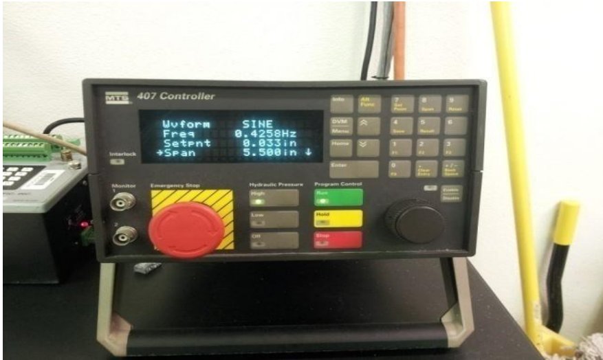
Figure 20 MTS 407 wave tank controller set to Wave Type II, .42 Hz, 5.5” Span
