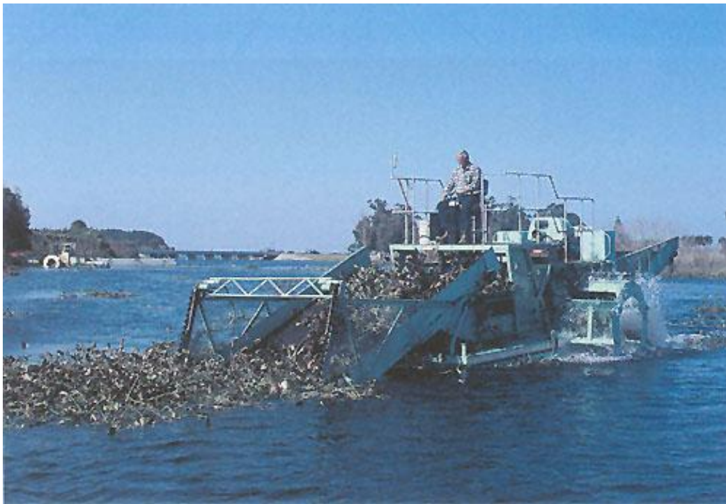
Figure 31 Water Hyacinth Harvester (University of Florida IFAS Extension, 2012)
