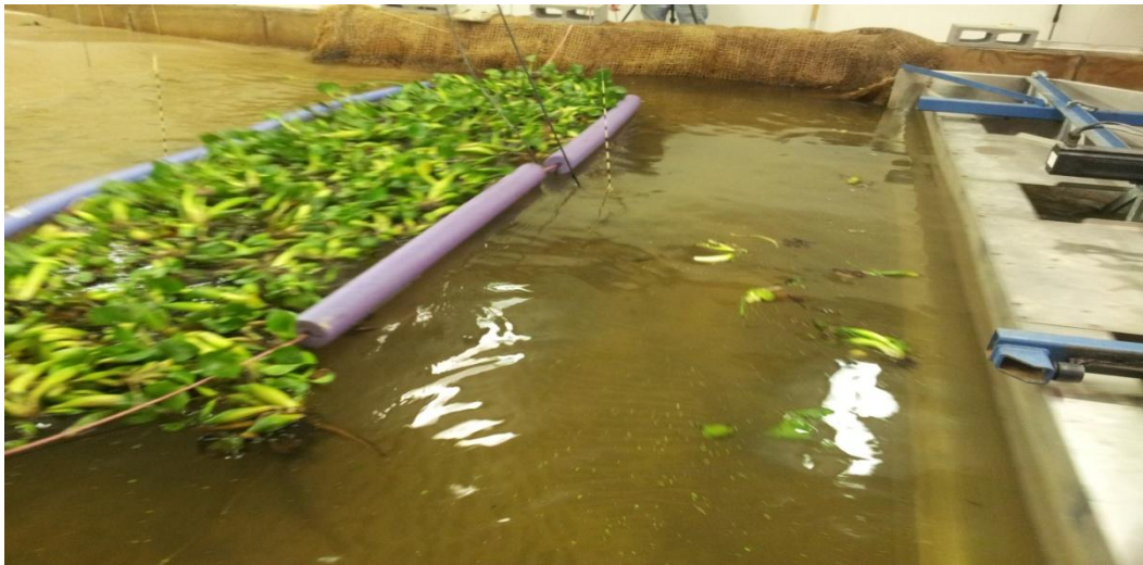
Figure 17 Booms hold plant biomass in place so that wave energy absorption can be observed
