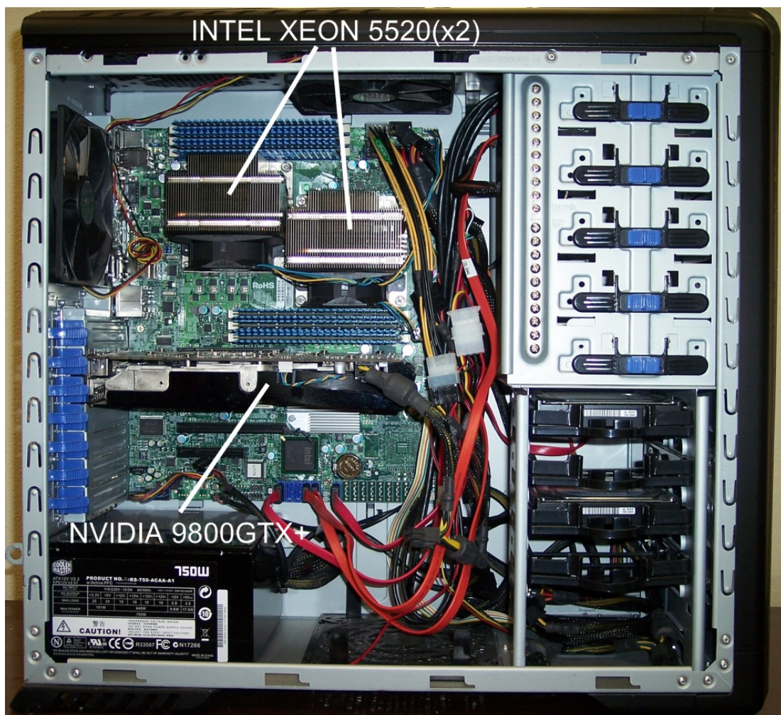
Figure 3-1. Test platform: Dual Intel Xeon 5520 CPUs and Nvidia 9800GTX+
