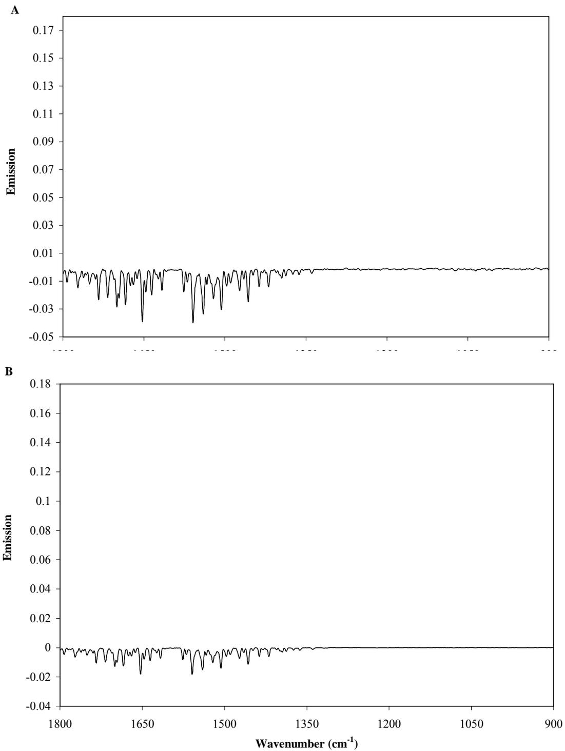
**Figure 40. FTIR reflection spectra of an (a) aluminum and a (b) stainless steel plate before *P. aeruginosa* biofilm formation.**
