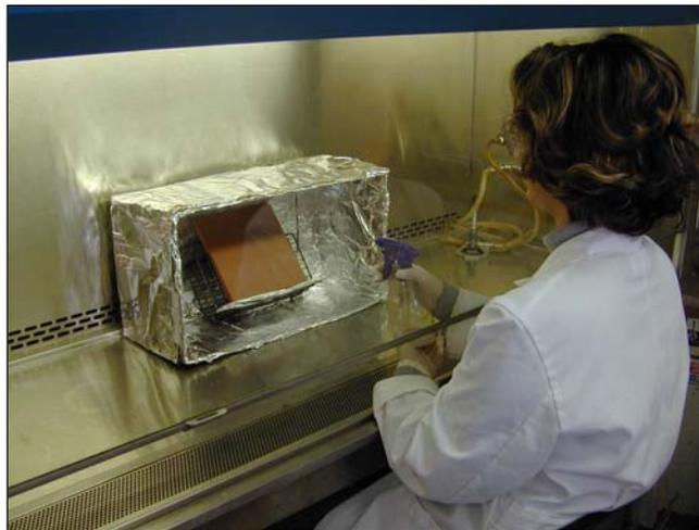
**Figure 14. Contamination of test materials with *Bacillus subtilis* spores.**
