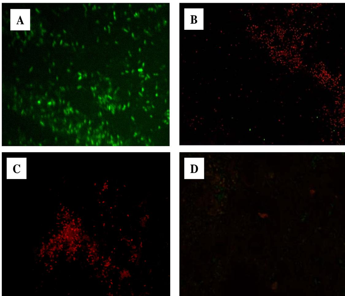
**Figure 39. Confocal scanning laser images of six days old *P.aeruginosa* biofilm on aluminum surfaces.** Bacterial cells (a) before and after treatment with biocidal complex (hydrogen peroxide: sodium hypochlorite) at a 1/10 ratio (2,500 ppm H<sub>2</sub>O<sub>2</sub>) for (b) 1 min, (c) 5 min and (d) 20 min. Images taken at 40 X and 63 X magnification.
