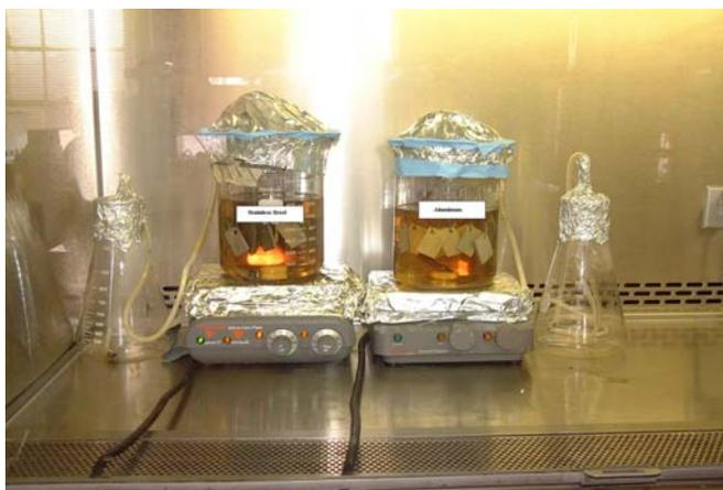
**Figure 6. Growth of *P. aeruginosa* ATCC 19142 biofilm on vertically suspended stainless steel and aluminum plates.**
