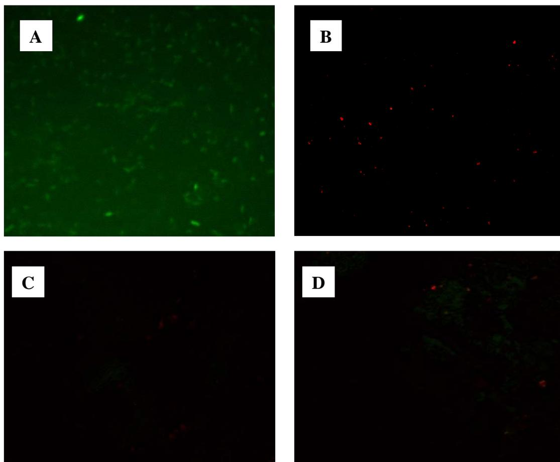
**Figure 38. Confocal scanning laser images of six days old *P.aeruginosa* biofilm on stainless steel surfaces.** Bacterial cells (a) before and after treatment with biocidal complex (hydrogen peroxide: sodium hypochlorite) at a 1/10 ratio (2,500 ppm H<sub>2</sub>O<sub>2</sub>) for (b) 1 min, (c) 5 min and (d) 20 min. Images taken at 40 X and 63 X magnification.
