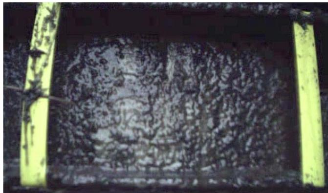
**Figure 15.** A section of a wash table covered with biofilm at Cora Texas mill, LA.
