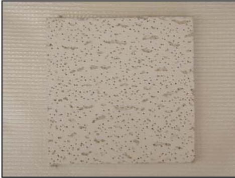
**Figure 10. Acoustic ceiling tile.**
