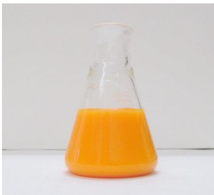
Figure 3.1. Colloidal Cu_2O mixture after wet chemical reduction.
