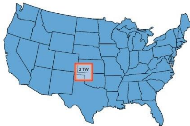
Figure 1.2. Representation of land requirement for solar panel to meet the energy demands in the United States. (Source: Lewis, N.S. 2007. "Powering the Planet." Engineering and Science No. 2, p. 22)
