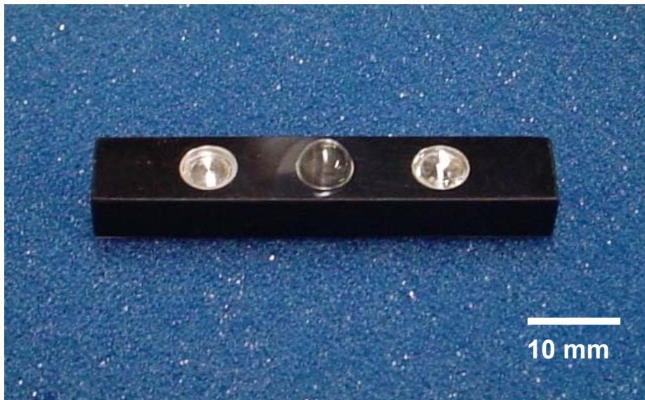
Figure 3.6. Calibration set for the calibration of contact angle measurement. The structure imitates the contact angles of 15.9^\circ , 90^\circ , and 39.6^\circ from the left.
