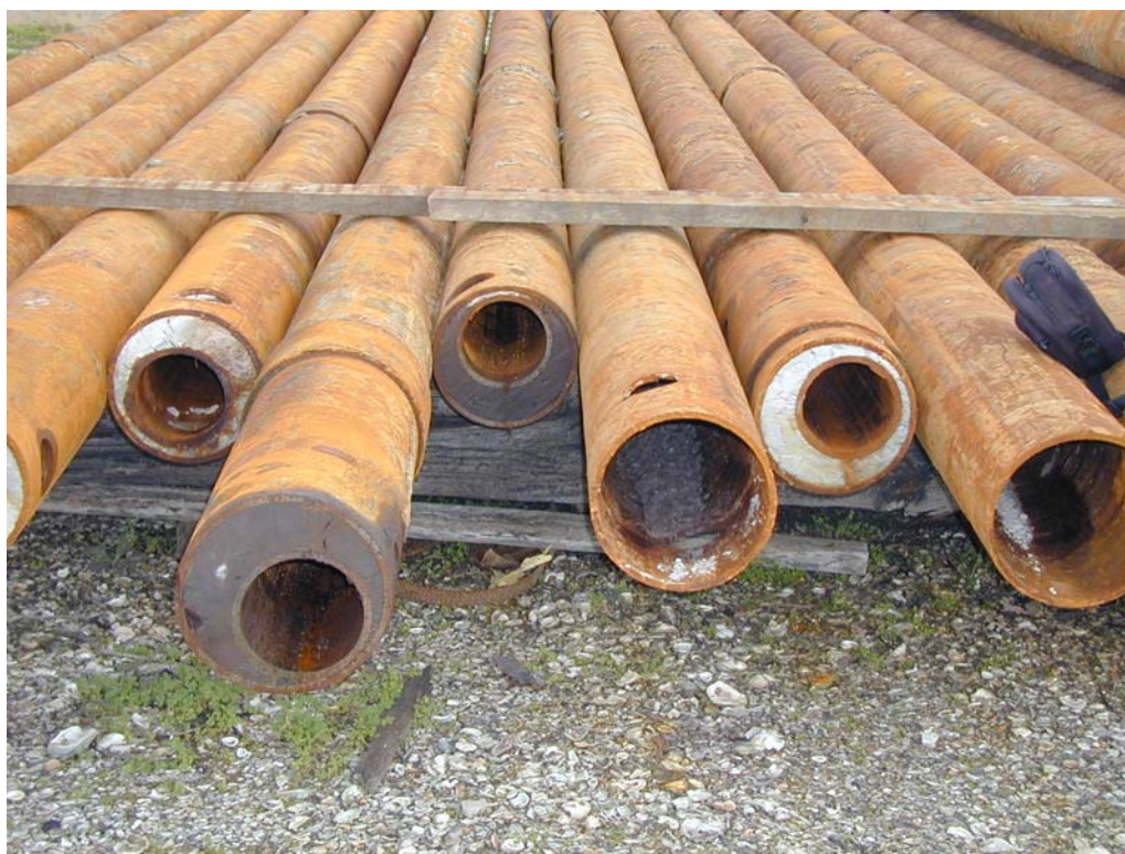
Figure 5-4: 7 and 10 \frac{3}{4} -in. Casing on the Rack after being Cut and Pulled
