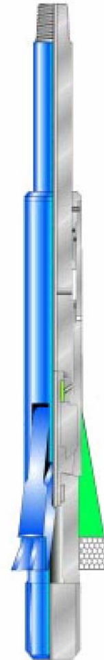
Figure 4-7: Lockomatic Section Mill used during 1999 Workover Program
