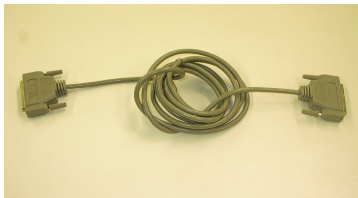
Figure A.9 A CEXP2DAS16-10 cable was used to connect EXP32 with the A/D board. The cable connects the A/D board from then rear of the PC. One end marked MUX was connected to EXP32 and other end connected the A/D board
