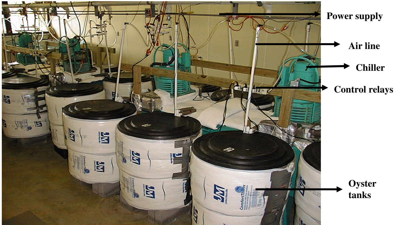
Figure 3.7 Photograph of the system developed at the LSU Aquaculture Research Station. All tanks were insulated using encapsulated fiberglass insulation to prevent heat loss.
