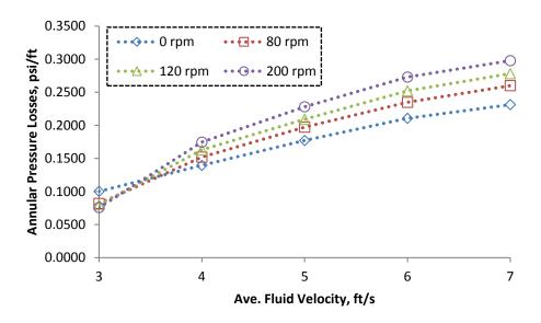
Figure 7-4: Annular pressure losses as function of fluid velocity and pipe rotation with particle injection rate of 0.105 kg/s
