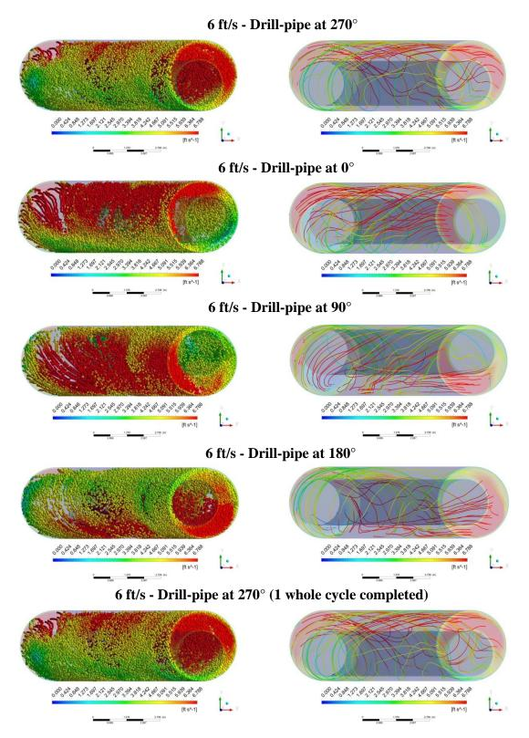
Figure 7-33: Trajectory of particles and 3D streamlines of fluid velocity for forward whirling [whirling speed: (+) 120 rpm, rotary speed: (+) 80 rpm] at 6 ft/s of fluid velocity
