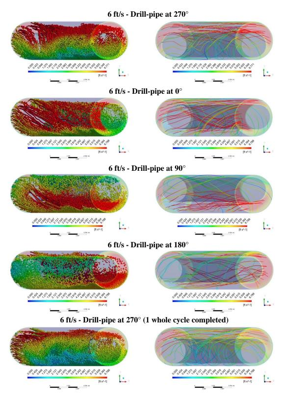
Figure 7-29: Trajectory of particles and 3D streamlines of fluid velocity for forward whirling [whirling speed: (+) 40 rpm, rotary speed: (+) 80 rpm] at 6 ft/s of fluid velocity
