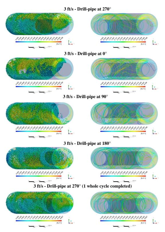
Figure 7-31: Trajectory of particles and 3D streamlines of fluid velocity for forward whirling [whirling speed: (+) 120 rpm, rotary speed: (+) 80 rpm] at 3 ft/s of fluid velocity
