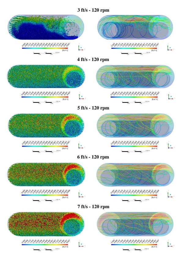
Figure 7-15: Trajectory of particles and 3D streamlines of fluid velocity for varying fluid velocity at rotary speed of 120 rpm
