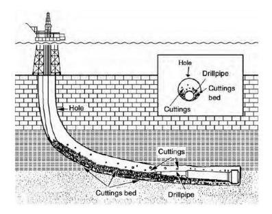
Figure 1-1: Schematic of cuttings bed build-up during directional drilling [2]
