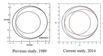
Figure 6-9: Forward Whirl with Forward Slip, Rotation Speed -2.2 Hz, Whirling Speed -3.3 Hz
