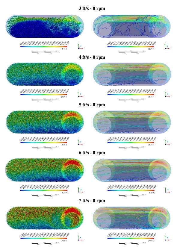
Figure 7-13: Trajectory of particles and 3D streamlines of fluid velocity for varying fluid velocity at rotary speed of 0 rpm
