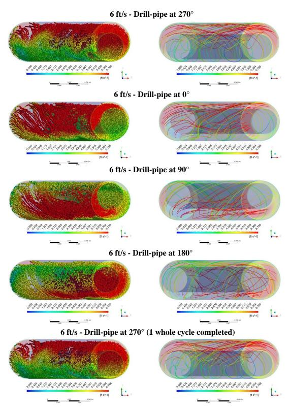
Figure 7-37: Trajectory of particles and 3D streamlines of fluid velocity for synchronous whirling [whirling speed: (+) 80 rpm, rotary speed: (+) 80 rpm] at 6 ft/s of fluid velocity
