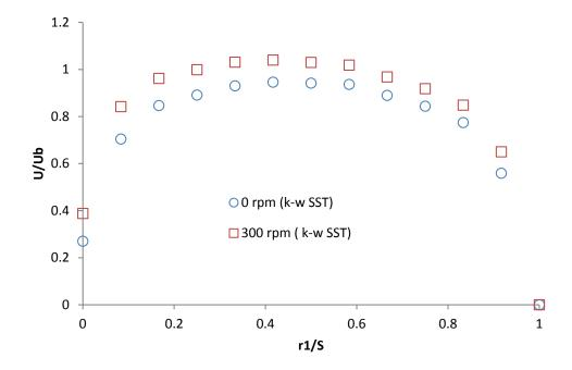
Figure 4-16: Comparison of axial velocity values normalized with bulk velocity with respect to the presence of the inner-pipe rotation for k-w SST turbulence model at Plane 1
