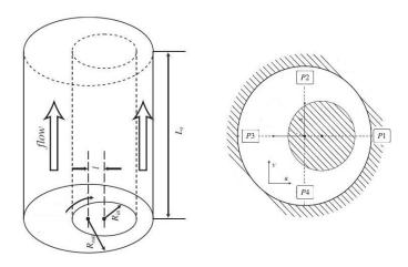
Figure 4-6: Geometric demonstration of computational set-up for eccentric annuli: Locations of the lines Plane 1 to Plane 4 (redrawn from Ninokata *et al.*, 2006)
