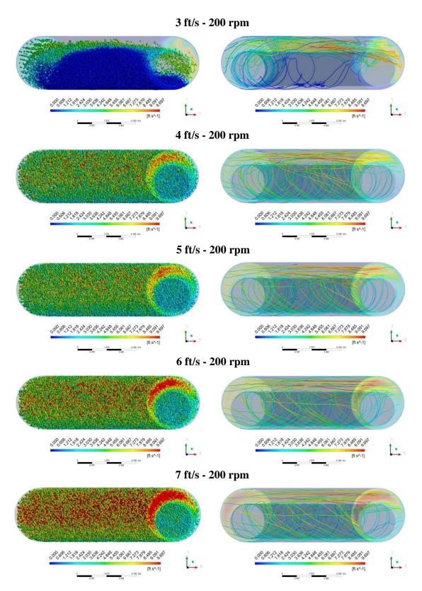
Figure 7-16: Trajectory of particles and 3D streamlines of fluid velocity for varying fluid velocity at rotary speed of 200 rpm
