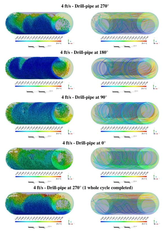
Figure 7-20: Trajectory of particles and 3D streamlines of fluid velocity for backward whirling [whirling speed: (-) 40 rpm, rotary speed: (+) 80 rpm] at 4 ft/s of fluid velocity
