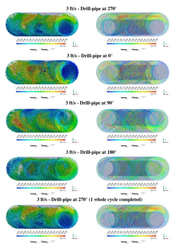
Figure 7-27: Trajectory of particles and 3D streamlines of fluid velocity for forward whirling [whirling speed: (+) 40 rpm, rotary speed: (+) 80 rpm] at 3 ft/s of fluid velocity
