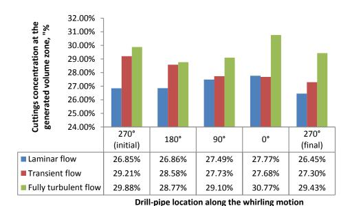
Figure 7-26: Cuttings distribution along the whirling rotary at the virtual region at backward whirl at 120 rpm
