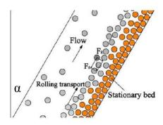
Figure 1-5: Rolling/sliding transport in inclined well [13]
