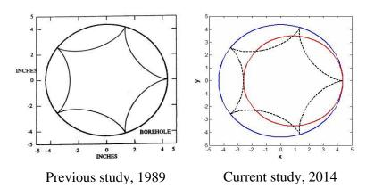
Figure 6-4: Backward Whirl, No Slip, Rotation Speed -2.2 Hz, Whirling Speed 8.8 Hz
