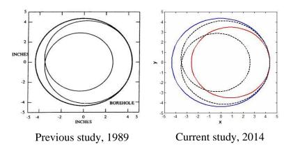
Figure 6-7: Forward Whirl with Slip, Rotation Speed -2.2 Hz, Whirling Speed -1.1 Hz
