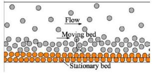
Figure 1-7: Rolling/Sliding transport in horizontal well [13]
