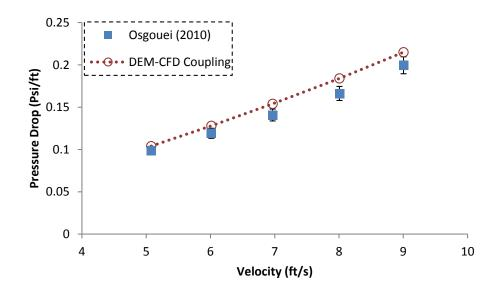
Figure 5-6: Comparison of annular pressure losses for cuttings-water multiphase flow in an eccentric horizontal annulus between the experimental and simulated data
