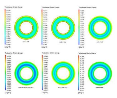
Figure A-3: Turbulence kinetic energy contours in a concentric annulus without inner pipe rotation for each turbulence model: (a) k-w SST, (b) k-w Stnd, (c) k-e Stnd, (d) k-e Realizable Stnd, (e) k-e RNG, (f) RSM SWF
