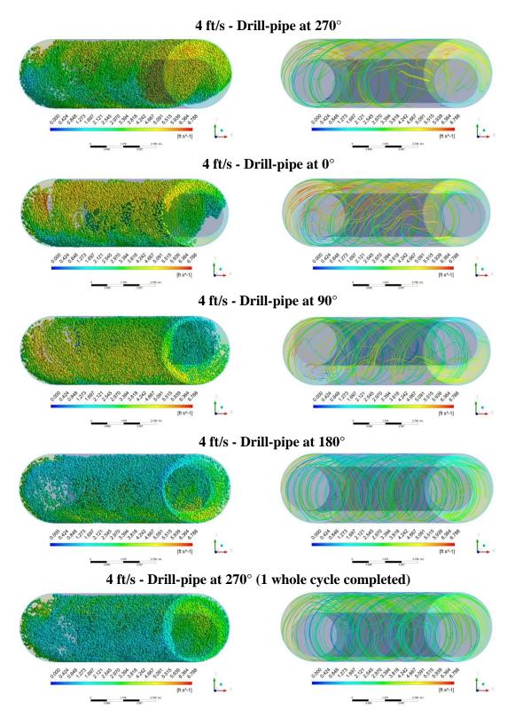
Figure 7-32: Trajectory of particles and 3D streamlines of fluid velocity for forward whirling [whirling speed: (+) 120 rpm, rotary speed: (+) 80 rpm] at 4 ft/s of fluid velocity
