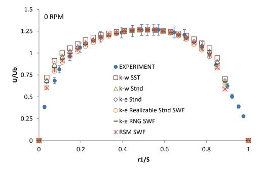
Figure 4-4: Simulated and experimental results for axial velocity profiles normalized with bulk velocity in the concentric annuli without inner pipe rotation
