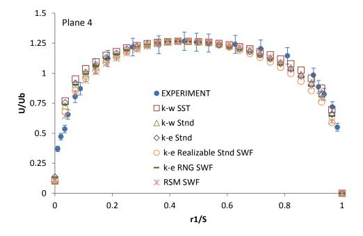
Figure 4-11: Simulated and experimental results for axial velocity profiles normalized with bulk velocity for Reynolds Number of 9300 in the eccentric annuli without inner pipe rotation at Plane 4
