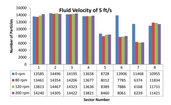
Figure 7-10: Particle distribution along sectors at fluid velocity of 5 ft/s with rotational speed 0 to 200 rpm
