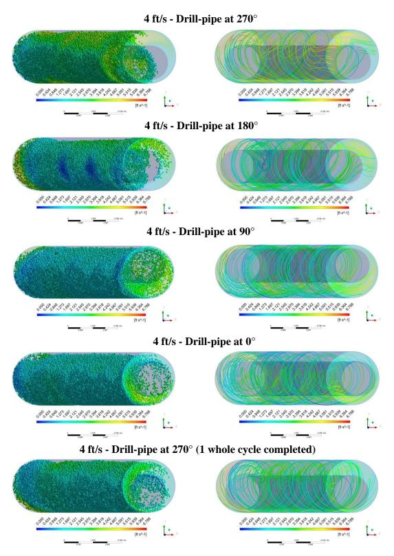
Figure 7-24: Trajectory of particles and 3D streamlines of fluid velocity for backward whirling [whirling speed: (-) 120 rpm, rotary speed: (+) 80 rpm] at 4 ft/s of fluid velocity
