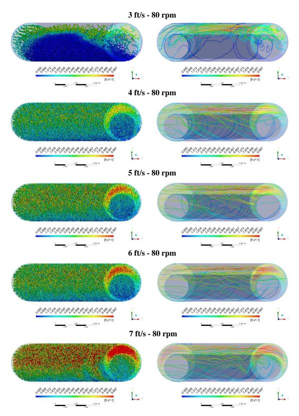
Figure 7-14: Trajectory of particles and 3D streamlines of fluid velocity for varying fluid velocity at rotary speed of 80 rpm
