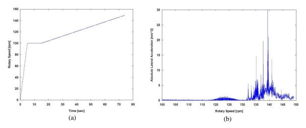
Figure 6-1: Analytical results for the occurrence of dynamic motion of the drill-pipe a) innerpipe rotary speed versus the time history, b) maximum lateral acceleration with respect to innerpipe rotary speed [71]
