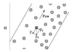
Figure 1-4: Suspension transport in inclined well (α represents deviation from vertical) [13]
