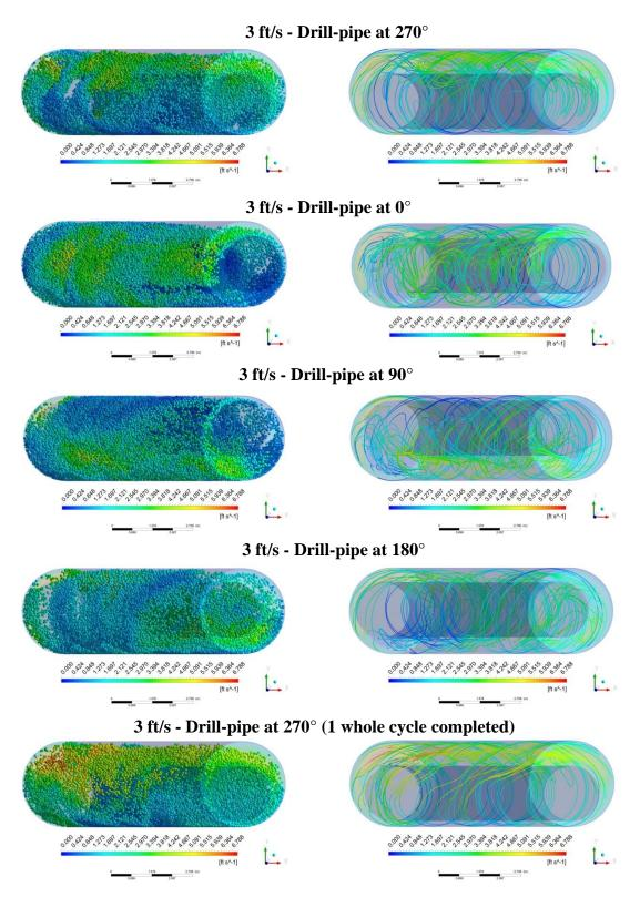
Figure 7-35: Trajectory of particles and 3D streamlines of fluid velocity for synchronous whirling [whirling speed: (+) 80 rpm, rotary speed: (+) 80 rpm] at 3 ft/s of fluid velocity
