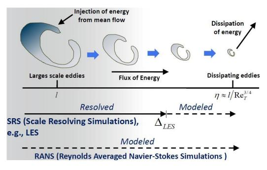
Figure 4-1: Dissipation of eddies in Energy Cascade [58]
