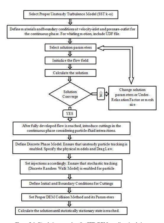
Figure 3-1: Simulation procedure for CFD-DEM coupling simulations
