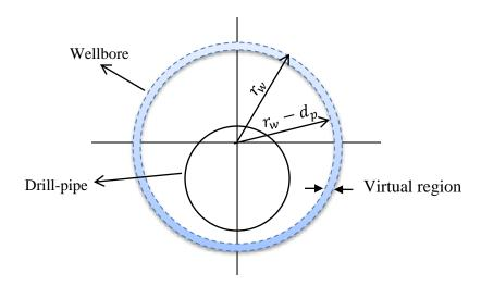
Figure 7-18: Wellbore cross-section for predicting presence of the plastering effect
