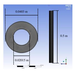
Figure 4-3: Concentric computational grid with inflation near wall
