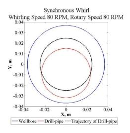
Figure 7-17: Snapshot of drill-pipe trajectory for 4 whole cycles at different mode of whirling of the drill-pipe in an eccentric horizontal well
