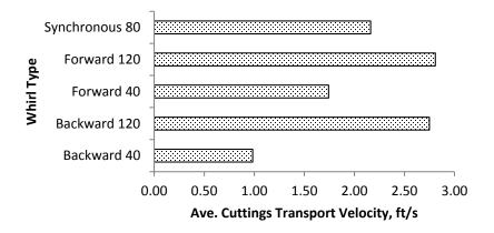
Figure 7-41: Average cuttings transport velocity as a function of whirling rotary at fluid velocity of 3 ft/s
