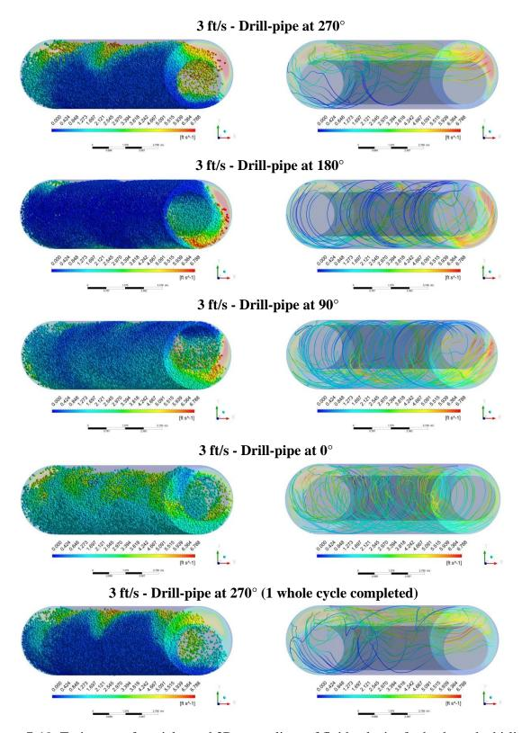
Figure 7-19: Trajectory of particles and 3D streamlines of fluid velocity for backward whirling [whirling speed: (-) 40 rpm, rotary speed: (+) 80 rpm] at 3 ft/s of fluid velocity
