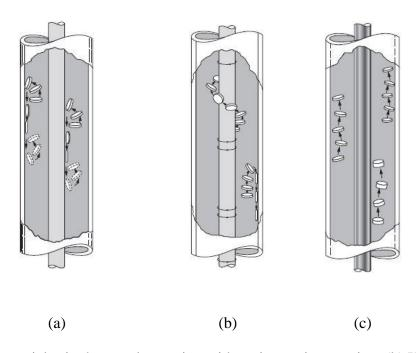
Figure 1-3: (a) Flat particles in the annular section without inner pipe rotation, (b) Helical motion of the flat particles with inner pipe rotation, and (c) Flat particles transported in turbulent flow without inner pipe rotation [12]
