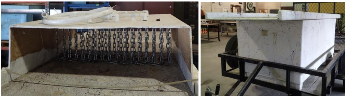
Figure 4 (a) Standard oyster washer typically used in Louisiana for on-shore shellfish washing. (b) The prototype on-board chilling unit.
