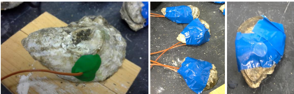
Figure 7 (a) A T-type thermocouple inserted into a live oyster and sealed with modeling clay. (b) Thermocouples secured with duct tape to ensure contact with the shell. (c) Smart Button attached to the outside of a live oyster using duct tape.
