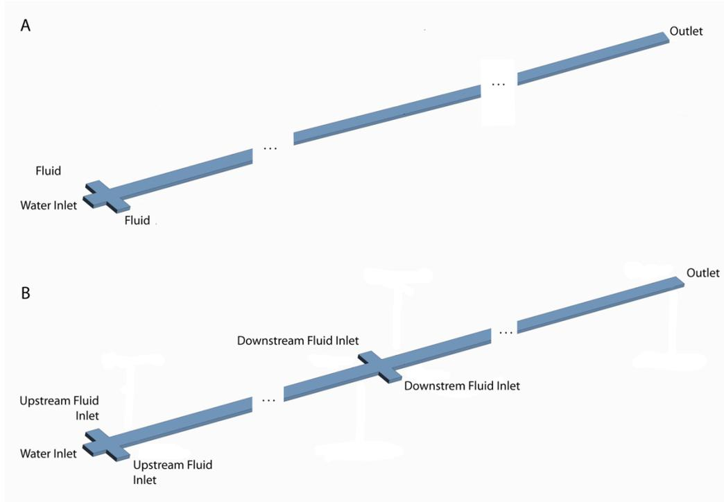
FIGURE 2: SCHEMATIC OF MICROCHANNEL GEOMETRIES. Renderings of microchannel domains constructed for numerical simulations of (A) single cryoprotectant cases and (B) cryoprotectant cocktail cases. Both geometries are identical with the exception that the cocktail geometry has a second set of inlets exactly half way down the length of the channel. The channels are 200  $\mu\text{m}$  in width, 50  $\mu\text{m}$  in depth, and 12.5 cm in length from the fluid junction at the main inlet.
