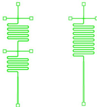
FIGURE 8: CHANNEL GEOMETRIES FOR FABRICATION. Straight T-Chan geometries modified to fit stand microscope slide blueprint.
