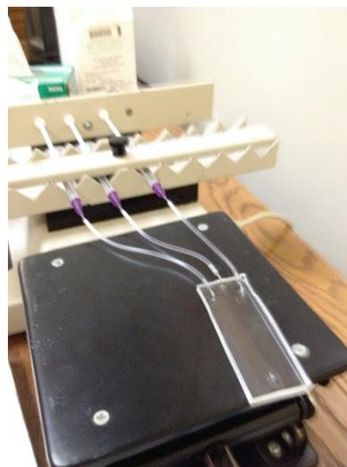
FIGURE 10: EXPERIMENTAL SET-UP FOR SINGLE CPA LOADING IN A MICROFLUIDIC DEVICE.
