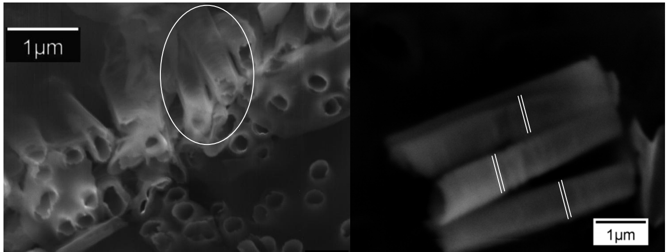
Figure 5.10 CoNiCu/Cu multilayered nanotubes: CoNiCu (-2 V) and Cu (-0.4 V)
