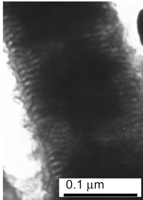
Figure 5.18 (a) TEM of CoNiFe/Cu wires (1 s alloy layer pulse)
