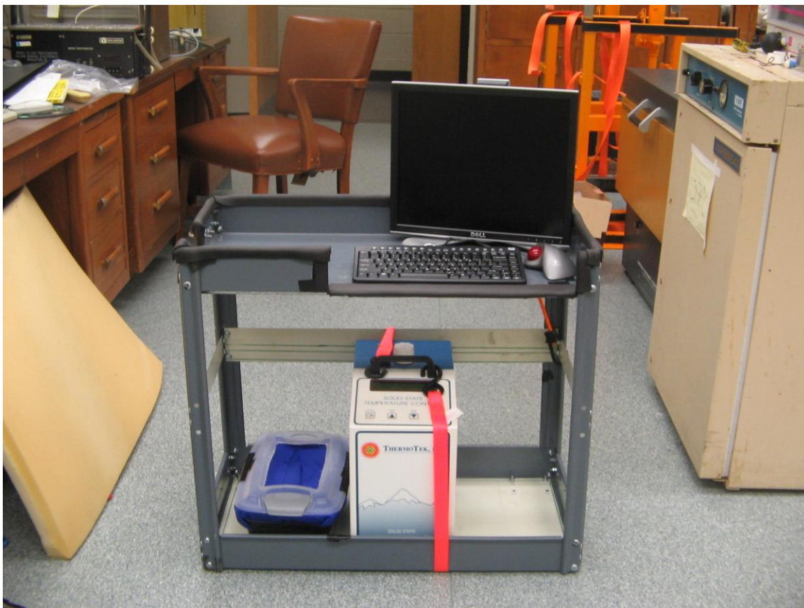
Figure E: Cart 2 holding the computer monitor, keyboard and trackball mouse. The water bath is placed in the bottom of the cart
